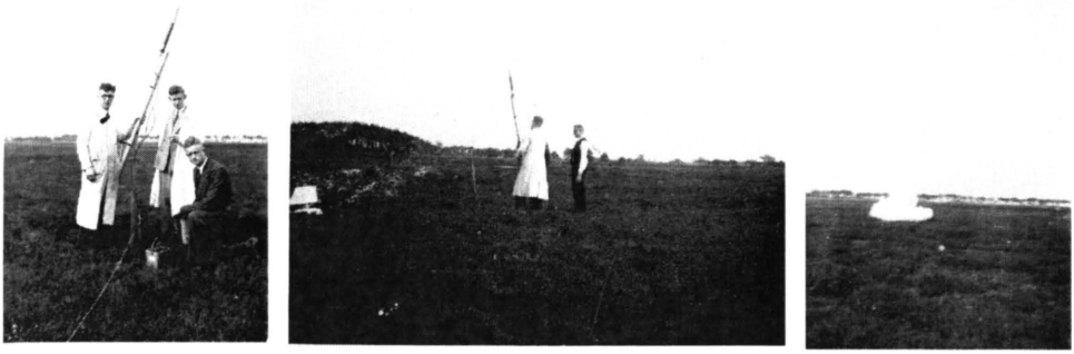
Figure 4-39,* 40 and 41†: Trial no. 34—Test rocket with a new charge—new design—now a D.R.P. patent—20 kg thrust—700 m altitude.
