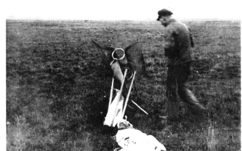
Figure 4-62 (right): Parachute got caught in the lower pointed tips of the steering panels and came down with the rocket that broke in the crash. Bad luck! Big ... Schwiegerhensen.§
