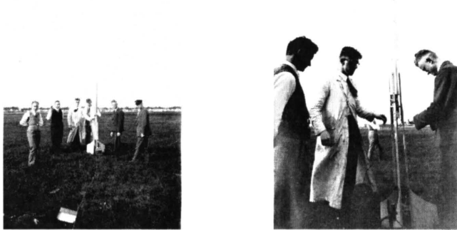
Figure 4-42‡ and 43§: Trial no. 32. 35–45 kg thrust—500 m altitude—weight = 8.5 kg – “without” guidance—(Rak II).
