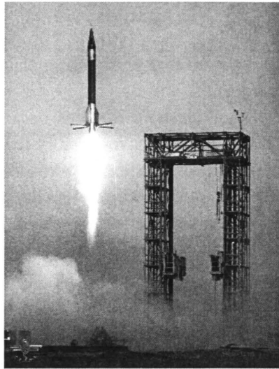
Figure 16–24: V50 launch: note the broken wire. [CERMA].
