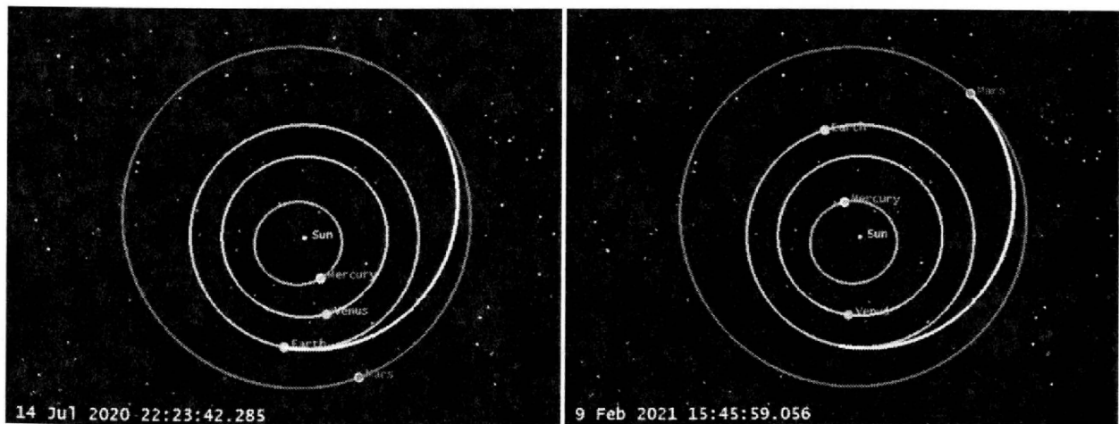
Figure 9. EMM's interplanetary cruise, with planets shown at the time of launch (left) and at the Mars arrival (right).
