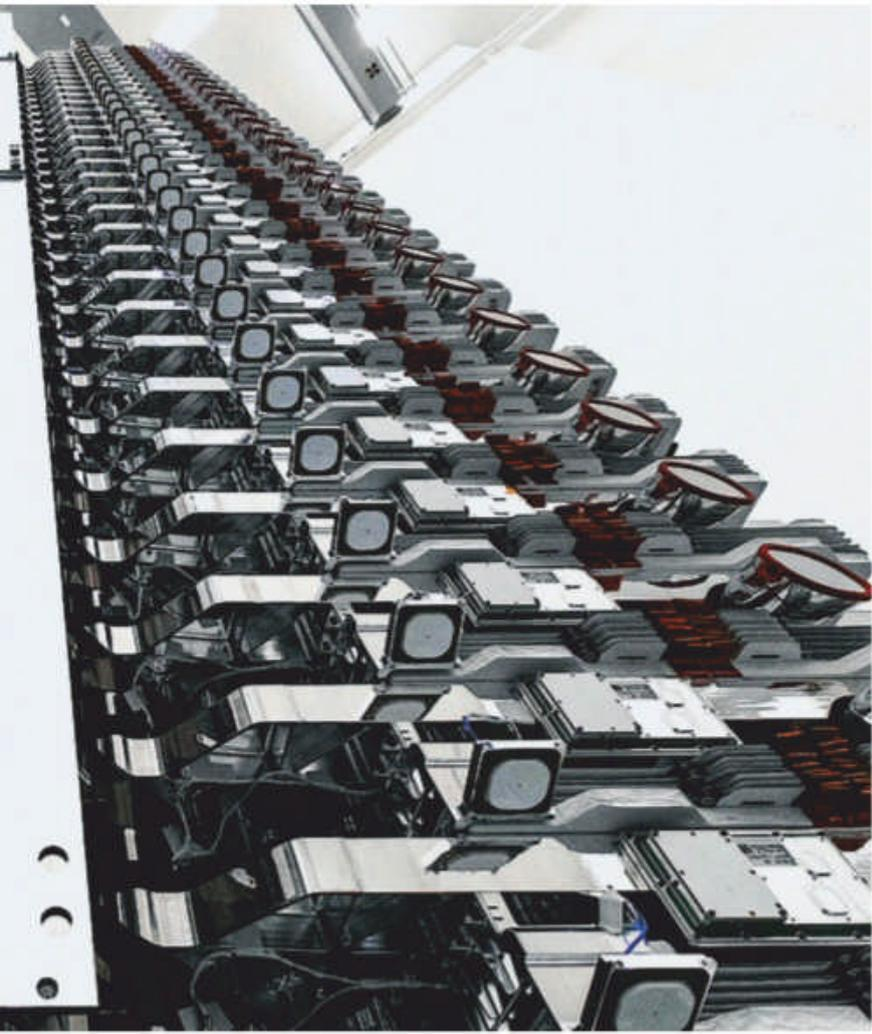
← A stack of Starlink comsats before they're loaded into a container and onto a rocket for the ride to low Earth orbit. SpaceX launches 60 of the 260-kilogram satellites at a time.
