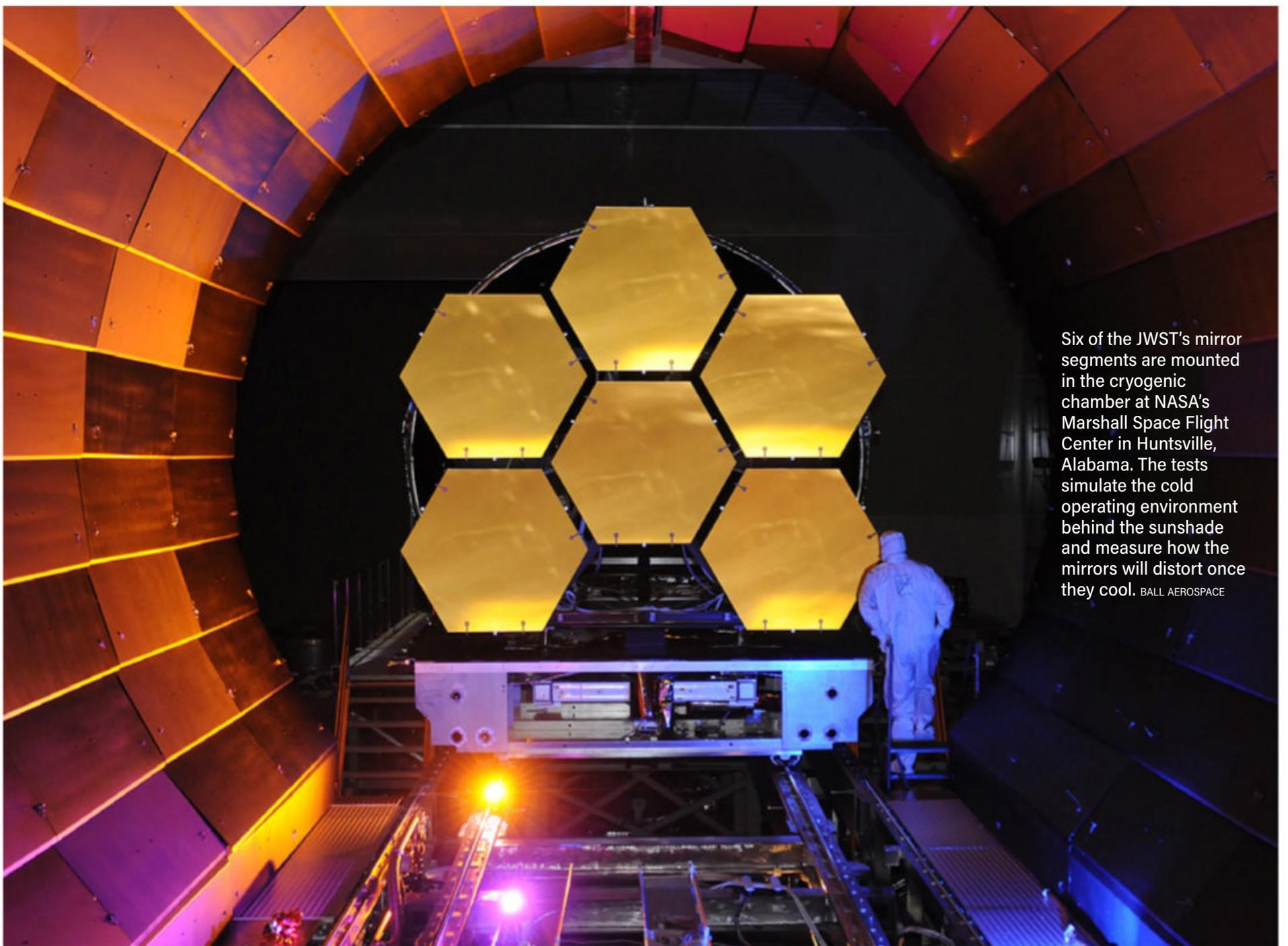
Six of the JWST's mirror segments are mounted in the cryogenic chamber at NASA's Marshall Space Flight Center in Huntsville, Alabama. The tests simulate the cold operating environment behind the sunshade and measure how the mirrors will distort once they cool. BALL AEROSPACE
