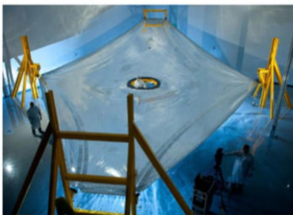
The Webb's sunshield consists of five layers, each made of a high-performance plastic film called Kapton and coated with aluminum and doped silicon. NORTHROP GRUMMAN
