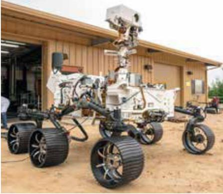
On September 4, while Perseverance was en route to Mars, JPL moved the rover's twin — a full-scale engineering model dubbed OPTIMISM (Operational Perseverance Twin for Integration of Mechanisms and Instruments Sent to Mars) — to its "Mars Yard" test area. Engineers can test rover commands and operations using OPTIMISM in an environment that simulates the Red Planet to better understand what Perseverance is experiencing on Mars. NASA/JPL-CALTECH
