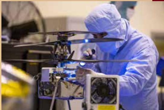
The experimental helicopter drone Ingenuity will become the first aircraft to take powered flight on another world. Though it won't be able to wander far — it will stay less than 0.6 mile (1 km) from the Perseverance rover to remain in wireless communication (right) — future drones could serve as more capable scouts. At left, Ingenuity receives its final inspection at the Kennedy Space Center in Florida before being mounted to Perseverance for its journey to Mars. NASA/JPL-CALTECH
