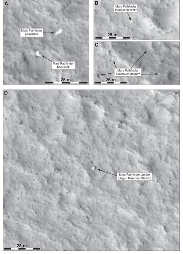
**Figure 160 Mars Pathfinder hardware on the surface.**The image is Mars Reconnaissance Orbiter HiRISE image PSP\_002391\_1995.
