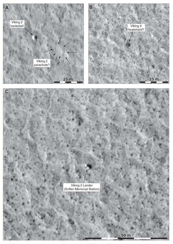
Figure 87 Viking 2 hardware on the surface of Mars, seen in HiRISE image PSP\_001501\_2280. The heatshield and parachute identifications are tentative.
