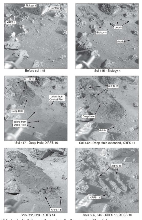
**Figure 98 Viking Lander 2 activities near Centaur, including the excavation of Deep Hole.**The last four stages are included here for spatial continuity but occurred in the following time period.
