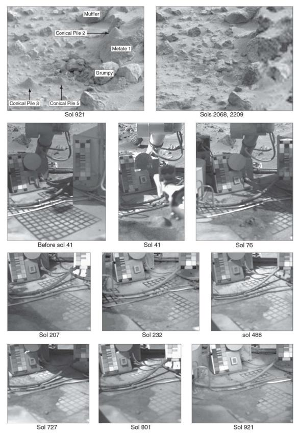
Figure 75 Changes observed near Conical Piles 2, 3 and 5 (top) and on the Viking Lander 1 spacecraft deck. Colour scale targets and the base of the high-gain antenna are visible beyond the gridded deck area.
