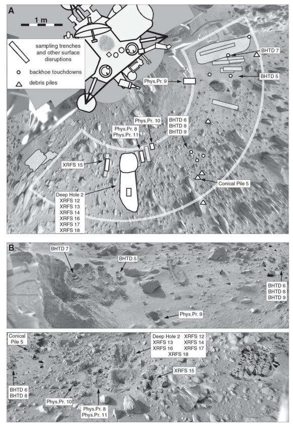
Figure 73 Viking 1 trenching activities up to the end of Surface Sampler operations.
