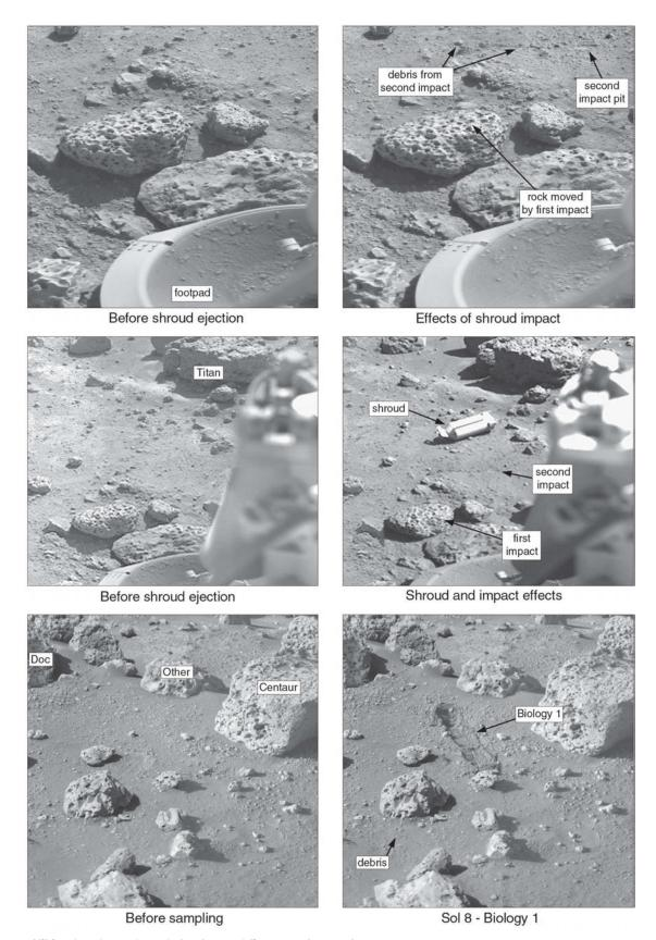
Figure 92 Viking Lander 2 shroud ejection and first sample trench.
