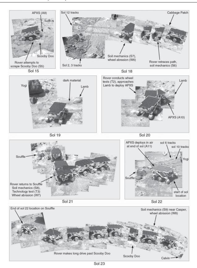
**Figure 169 Sojourner activities (continued from Figure 168)**. For scale in these figures, Sojourner is 63 cm long, 48 cm wide and its body is 28 cm high.
