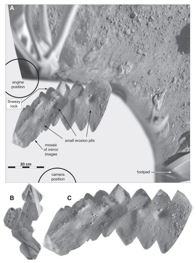
**Figure 106 A:** The immediate foreground of Viking Lander 2. The area mapped is roughly 1 m wide, with north at the top. **B:** A mosaic of images taken with an arm-mounted mirror to show the footpad temperature sensor. **C:** A mosaic of images taken using another mirror, showing engine erosion under the lander. Its approximate location is shown in (A), where small pits dug by the engine exhaust are indicated.
