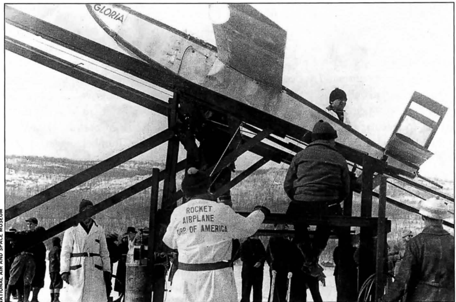
Loaded with thousands of letters, Gloria , a liquid-fueled rocket glider, is set to take off from a launch ramp at frozen Greenwood Lake, N.Y., in February 1936. It fizzled.
