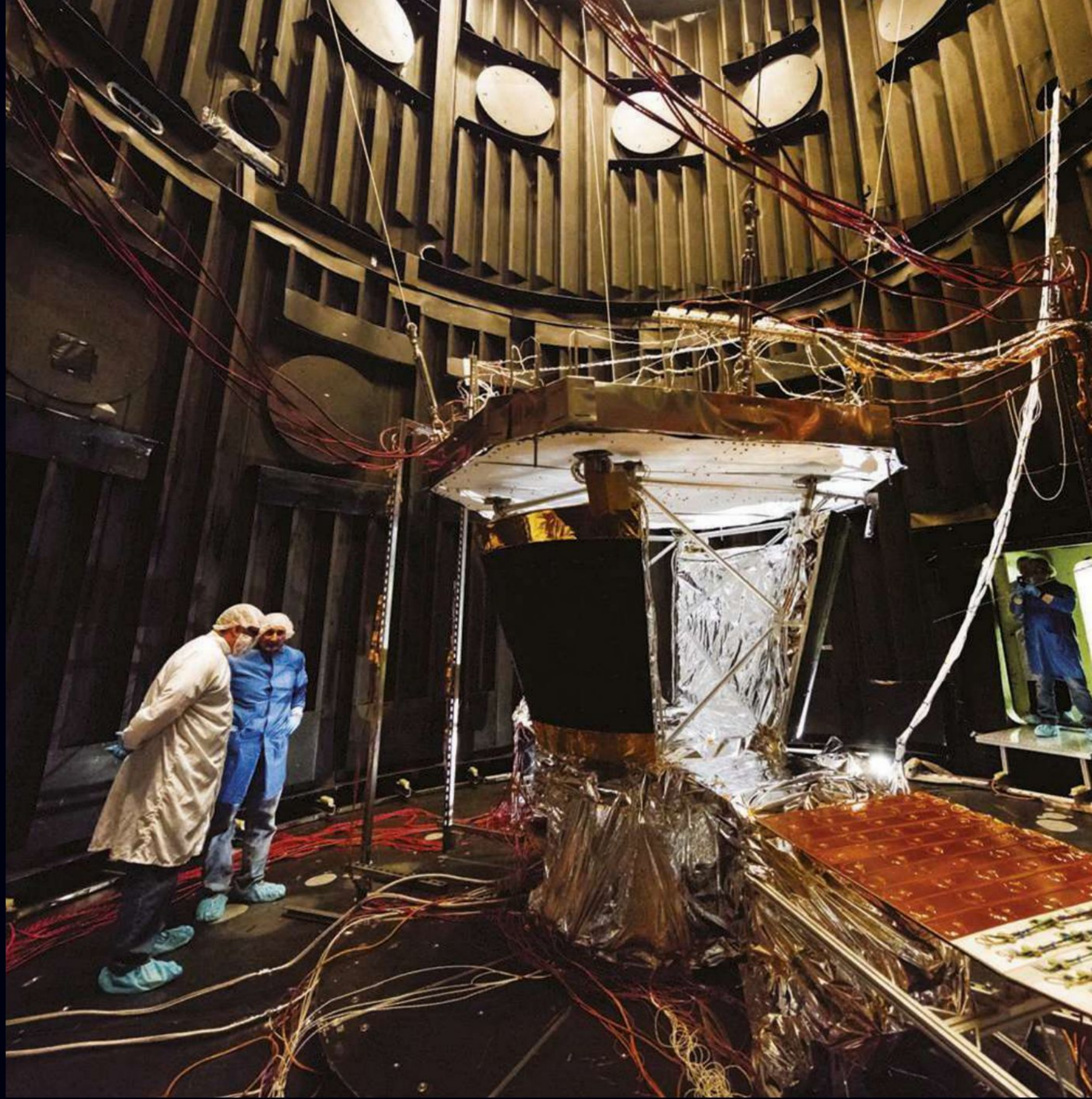
The solar array of the Parker Solar Probe undergoing thermal tests
