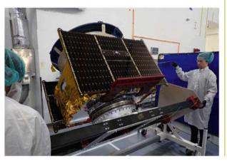
LEFT The main unit of the Varda W-1 mission under construction (the automated drug manufacturing capsule is upside-down at the top, between the solar panels)
