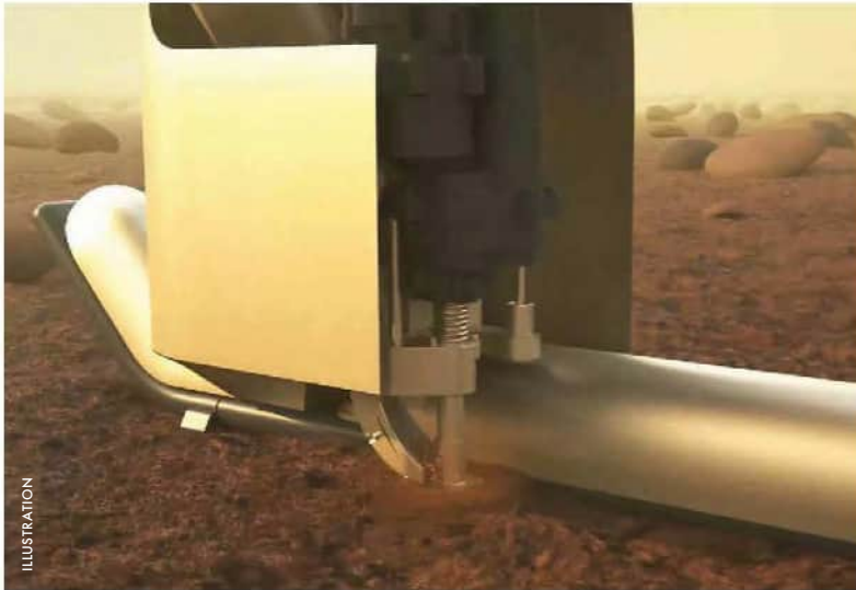
▲ When it lands, Dragonfly will fire up DrACO (Drill for Acquisition of Complex Organics)
