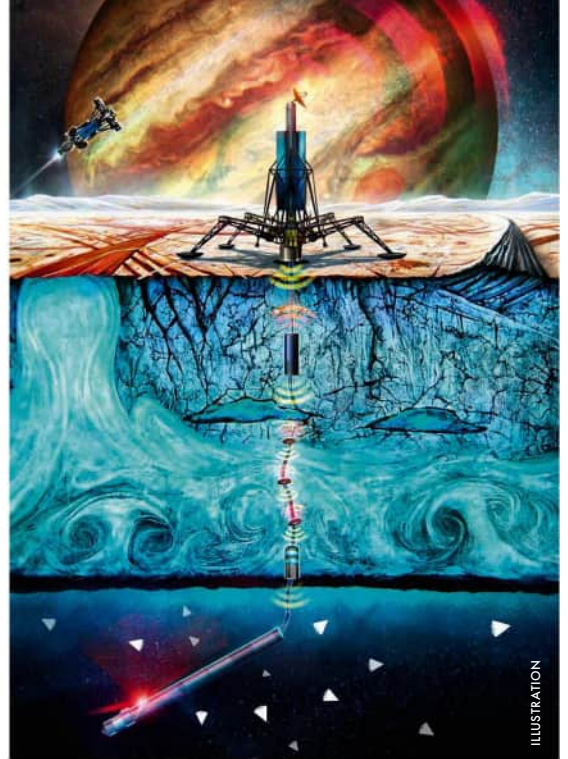
▲ Plans are under way for landers that melt through the miles of ice and release cryobots to study the oceans
