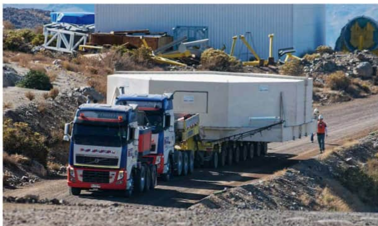
▲ Telescope components, like the huge 8.4-metre mirror shown here, had to be carefully transported up Cerro Pachón mountain
