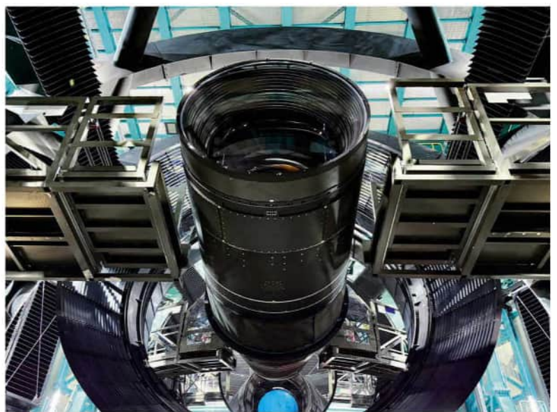
▲ Left: Rubin's 3.5-metre secondary mirror directs light from the primary onto the massive camera
