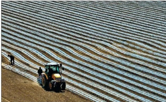
An autonomous-driving tractor pulls a wheat seeder in Zhangye, Gansu province, with the help of the Beidou Navigation Satellite System. WANG JIANG / FOR CHINA DAILY
