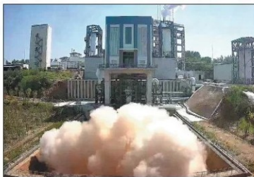
The ignition test of the new type of rocket engine designed to propel the third stage of the Long March 10 rocket is carried out at a newly built engine test facility in Beijing, PROVIDED TO CHINA DAILY.
