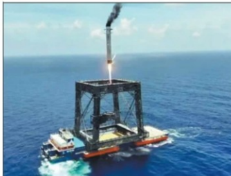
A video grab shows a platform mounted on the recovery ship Linghangzhe successfully capturing the first-stage booster of the Long March 10B carrier rocket on Friday. CCTV
