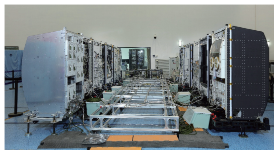
Fig. 1 Part of science experiment racks in Wentian and Mengtian are being tested on the ground
