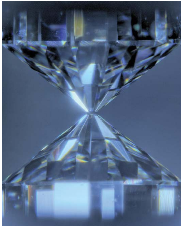
Diamonds are one of the hardest materials on Earth, and scientists can use them to compress iron to pressures inside Earth’s core. Credit: Kei Hirose
