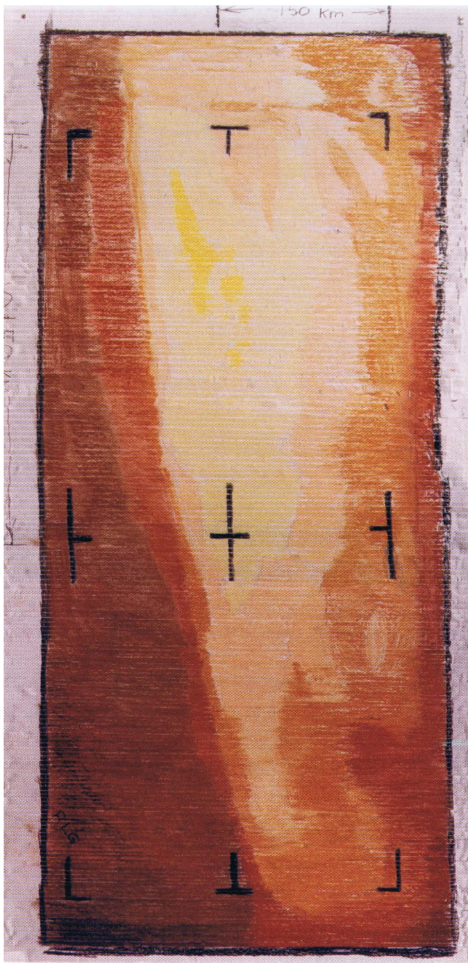
Plate 2. The initial version of Mariner 4 Picture Number 1 — the first close-up photograph of another planet ever taken. With a telemetry transmission rate of 8.33 bits per second, the 22 recorded photographs required four days to be sent back to Earth. As a communications dropout had occurred close to the moment of encounter, it was not known whether any pictures had actually been recorded, so the Mariner Product Manager directed that this picture be assembled in real time as the data came in. The numbers representing the brightness of each pixel in the picture were printed out in a vertical column on a strip of adding-machine tape by a computer at JPL. As the data from each scan line were completed, technicians cut the paper strip and pasted it onto a plywood sheet, overlapping the strips so as to produce one large 200 \times 200 matrix of numbers. Using colored chalk, they produced a kind of false-color contour map of the brightness of this historic picture. For many years it hung in the administration building at the laboratory, but recently it was moved into the Space Flight Operations Facility. See text p. 78.
