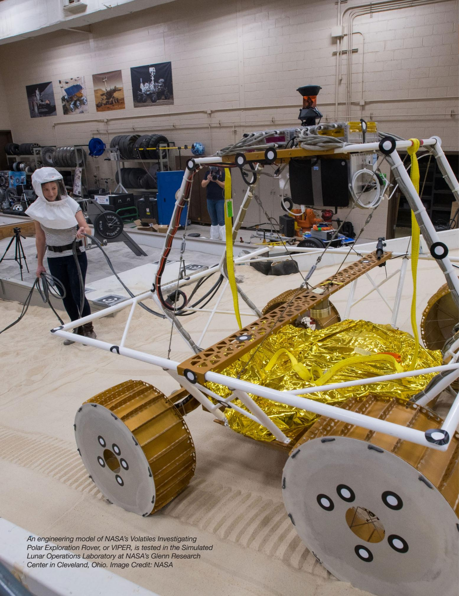
An engineering model of NASA's Volatiles Investigating Polar Exploration Rover, or VIPER, is tested in the Simulated Lunar Operations Laboratory at NASA's Glenn Research Center in Cleveland, Ohio. Image Credit: NASA
