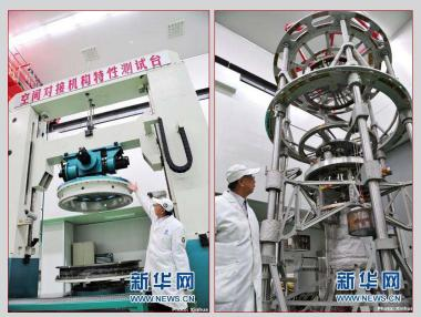
left: The Space Docking Characteristics Test-Bed. credit: Xinhua right: The Space Docking Thermal Vacuum Test-Bed. credit: Xinhua
