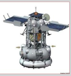
Graphic of the Phobos-Grunt spacecraft design. The Yinghuo 1 satellite is visible in the middle part of the Phobos-Grunt truss structure. credit: Lavochkin
