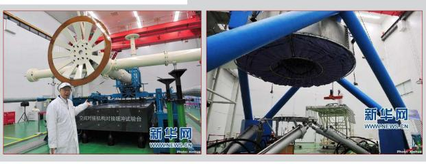
Each latch is able to provide a tightening force of 3 tonnes and each spring has pushing force of hundreds of Newtons. Five controllers, 18 electrical or electromagnetic actuators, 118 sensors, 291 gears, 759 bearings, 11,000 fasteners and nearly 10,000 other components work together to complete a docking operation.
