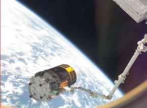
once the chaser spacecraft has delivered the capture interfaces of the chaser into the reception range of those of the target vehicle within the constraints of:
