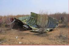
Debris of Shenzhou 8 fairing on ground. A high-altitude escape motor can be seen in this picture. (Internet photo)
