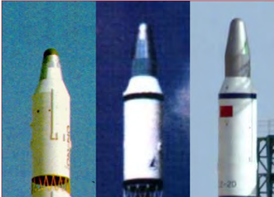
FSW satellite launch configuration comparison (left to right: FSW-0/1, FSW-2, FSW-3). (credit: Chinese Internet, Go Taikonauts!)
