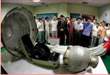
Debris of China's first recoverable satellite launched and recovered in 1975. Film canister, retro motor and the parachute can be seen. (credit: Chinese Internet)
