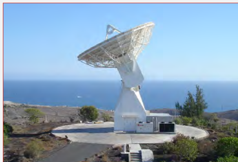
ESA's 15 m antenna in Maspalomas on the Canary Island of Gran Canaria. The dish operates for arriving signals in S- and X-Band and transmits radio waves in S-Band. (Credit: ESA)
