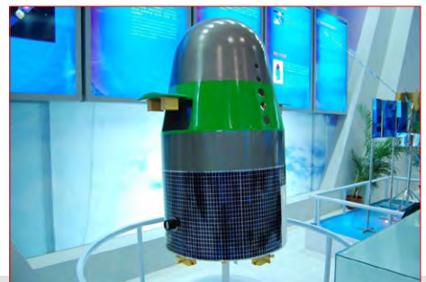
A model of the future recoverable satellite in display at the Zhuhai Air Show 2010. The new design has a large re-entry capsule and solar cells at the exterior of the instrument module. (credit: Chinese Internet)
