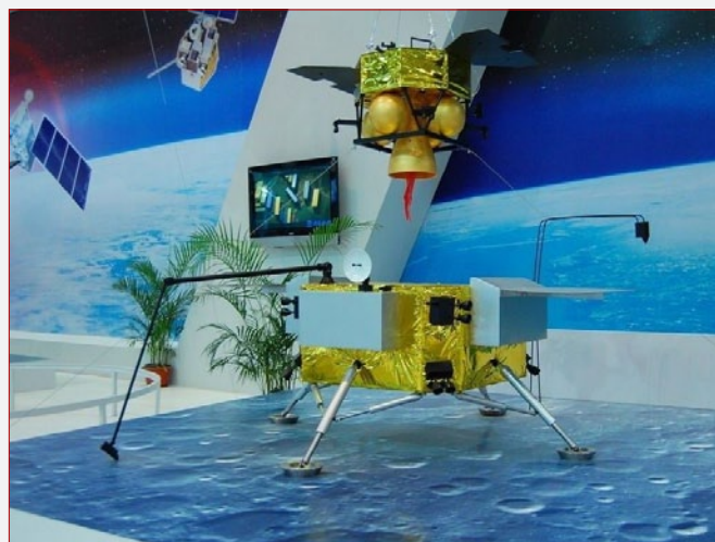
Model of the Chang'e 5 lunar sample return vehicle. Note its lander is almost identical to that of Chang'e 3. (credit: Chinese internet)
