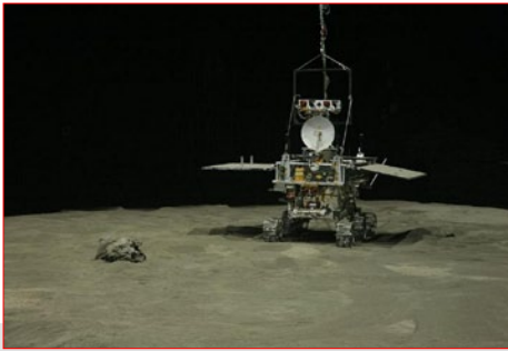
Yutu in indoor field-testing. It was suspended to simulate lunar gravity. (credit: Xinhua)
