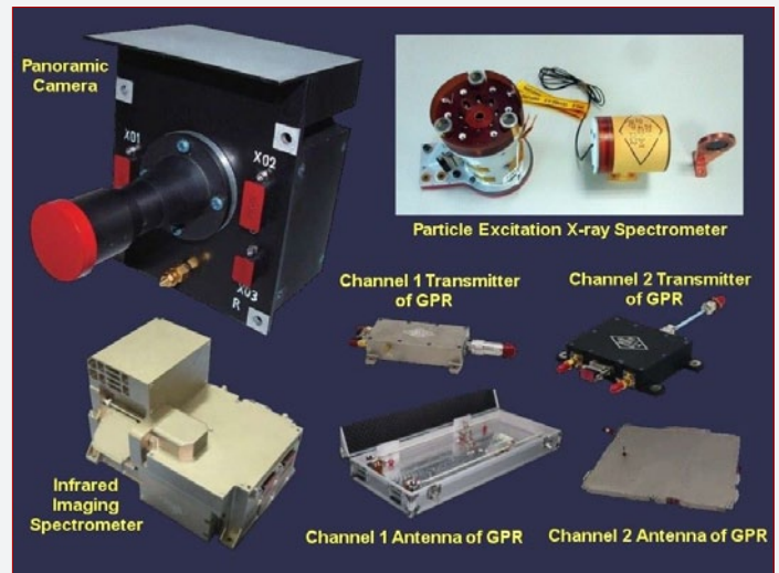
Payloads on the Chang'e 3 rover (credit: Go Taikonauts!/CAS)
