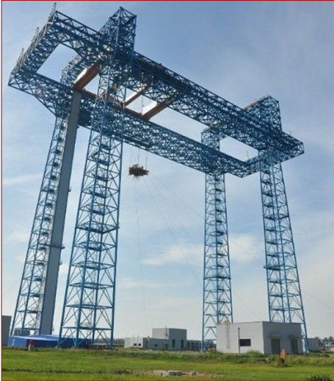
The drop-tower designed to test lunar descent and landing. (credit: Chinese internet)
