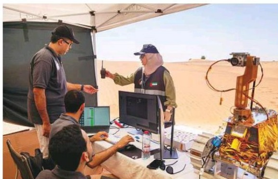
Rashid Rover can climb over an obstacle up to 10cm tall and descend a 20-degree slope.
