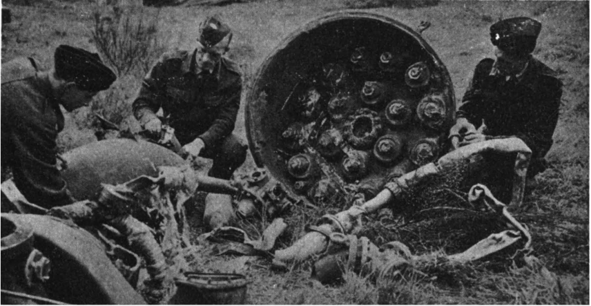
Fig. 2 The forward end of the jet unit showing 18 jets and parts of the V2.
