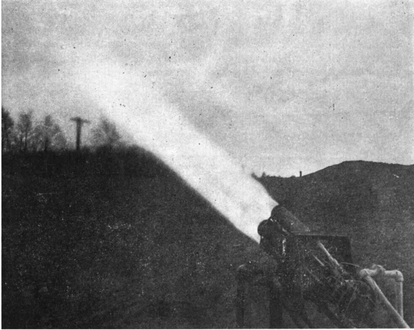
1500 N4C ROCKET ENGINE OPERATING AT 30° INCLINED POSITION.
