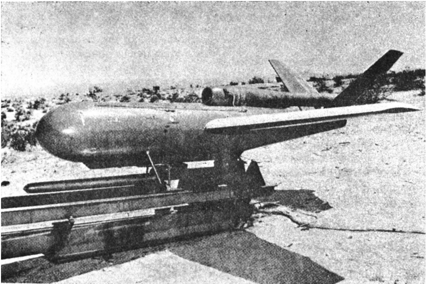
KDD-1 Target Drone, a remote radio-controlled pilotless aerial target, powered by one McDonnell pulsejet engine, and designed primarily for use as an anti-aircraft gunnery training target.
