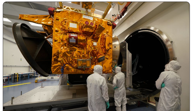
EMM engineers prepare the Hope Probe for environmental testing in LASP's new thermal vacuum chamber. (Courtesy Emirates Mars Mission)
