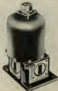
tion of 40 db. Maximum switching time is .25 sec. for 240° operation and .15 sec. for 120° operation. The universal switch operates at 3 amperes maximum at 28 vdc nominal and employs R.F. and pressurized fittings built into the switch, giving up to 20 lbs. of pressurization throughout.
