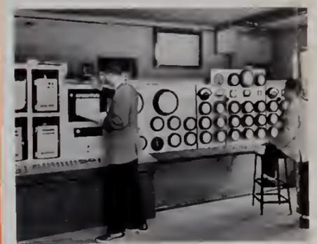
View from east of full-scale environmental qualification test of 1000 GPM RP Fuel Transfer system.
