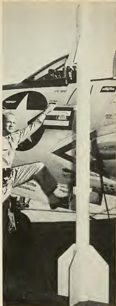
Bird is 4½ inches in diameter and 9 feet long. Current kill rate is 7 out of 10.
