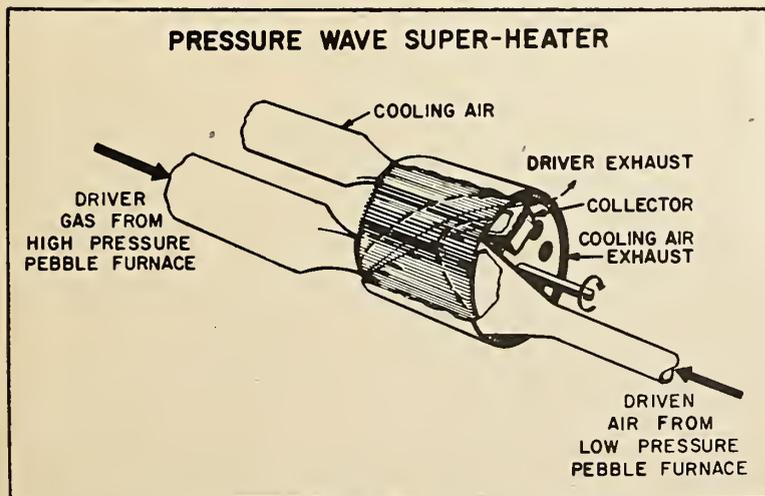
Diagram of a pressure wave super-heater such as that employed to extend the period of test conditions in a shock tube. This is typical of AFOSR-supported research programs.
