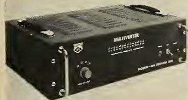
developed by Packard-Bell Computer Corp. subsidiary Packard-Bell Electronics Corp. Conversions are said to be provided at better than 0.01% and at speeds in excess of 15,000 per sec. for analog to digital and 300,000 per sec. for digital to analog conversion.
