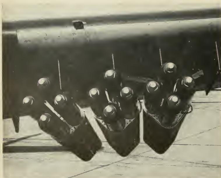
*ZUNI* is folding fin, solid propellant rocket, designed for fighter and attack-type aircraft, for air-to-air and air-to-surface attack. Expendable launcher holds four rockets.
