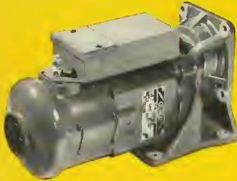
**Type:** D-751 DC Motor. **Weight:** 20 lbs. **Duty Cycle:** 5.2 hp at 2100 rpm (intermittent) on 26 volts DC; 3.5 hp at 2200 rpm (continuous) on 26 volts DC. **Meets Military Specification MIL-M-8609.**
