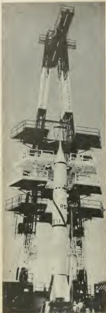
Army's REDSTONE missile in its servicing station at Patrick Air Force Base, Cape Canaveral, Fla., is being readied for test launching out over the Atlantic Ocean.
