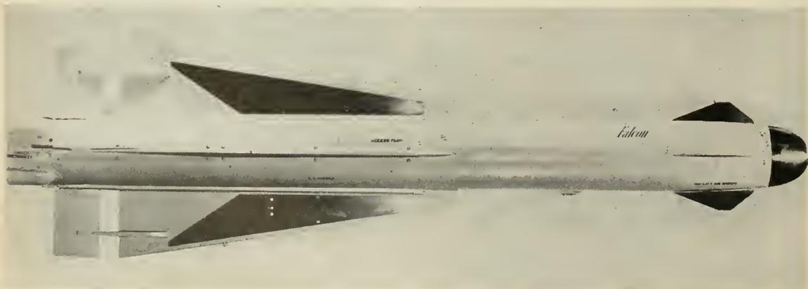
The air-to-air FALCON is the smallest guided missile in production. Slightly over 6 feet in length and weighing 110 pounds, it is powered by a Thiokol solid propellant propulsion unit. GAR-1D FALCON (above) incorporates aerodynamic improvements over earlier model.
