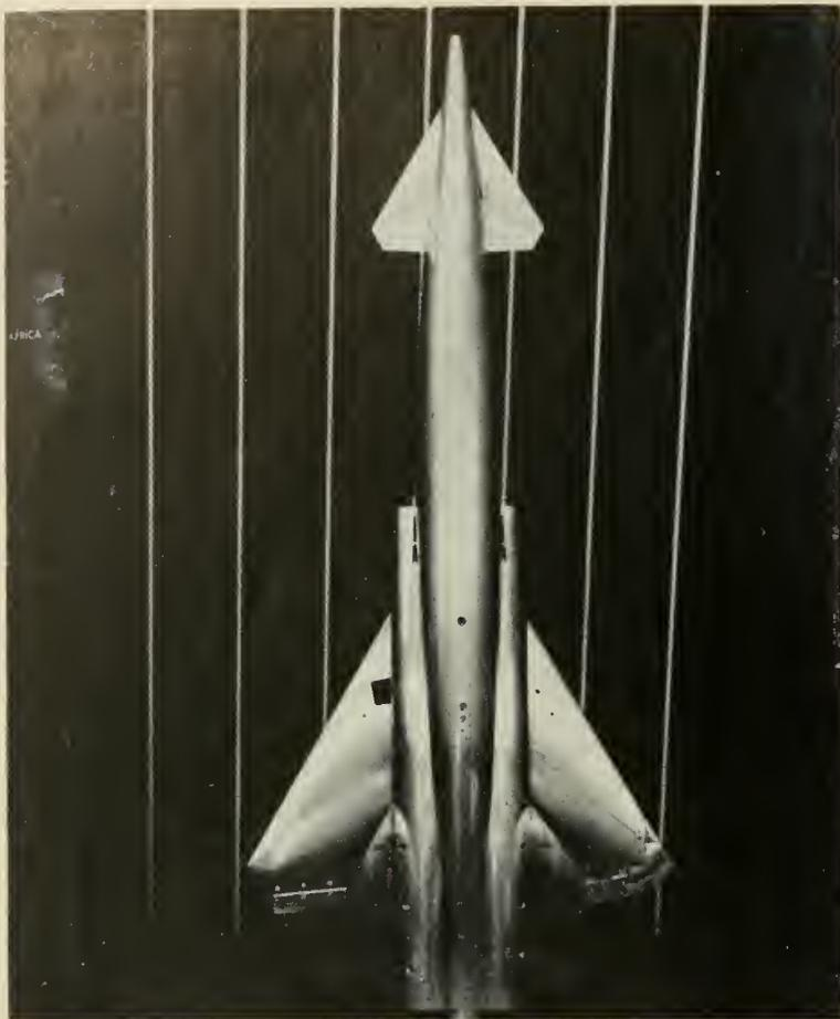
The fine detail of this large-scale wind-tunnel model of North American Aviation's NAVAHO test vehicle, the X-10, is a good example of the knowhow needed for missiles.
