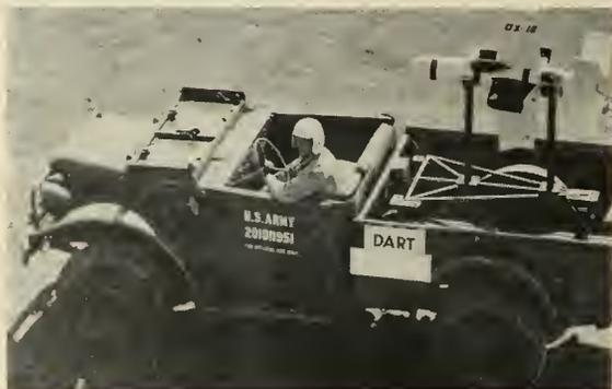
The highly mobile DART is shown on weapons carrier-launcher.
