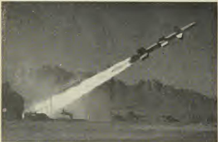
TALOS, boosted by solid propellant rocket, gathers speed as it roars from launcher. It will lock on target and when within lethal range a proximity fuse detonates the warhead.
