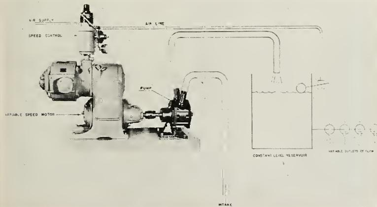
Variable flow rate pump-motor set designed specifically for pilot plant, laboratory or process work where controlled and varying rates of flow of corrosive fluids and abrasive slurries are required is being marketed by Vanton Pump & Equipment Corp.
