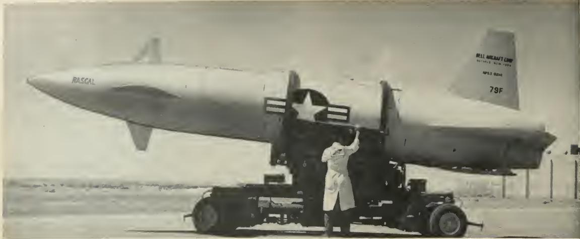
The GAM-63 *Rascal* is a liquid-propelled air-to-surface rocket missile under development for the Air Force by the Guided Missiles Division of Bell Aircraft Corp.
