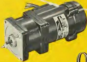
**Type:** C-1874 400 cycle 3 phase AC Motor and Clutch. **Weight:** 4.5 lbs. **Voltage:** 200 volts. **Output:** 650 watts. **Intermittent duty:** 12,000 rpm. **Meets Military Specification MIL-M-7969A (ASG).**
