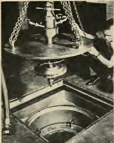
Impeller mounted on test arbor at Alcoa laboratory. Part will be spun until it flies to pieces in "whirl pit."
