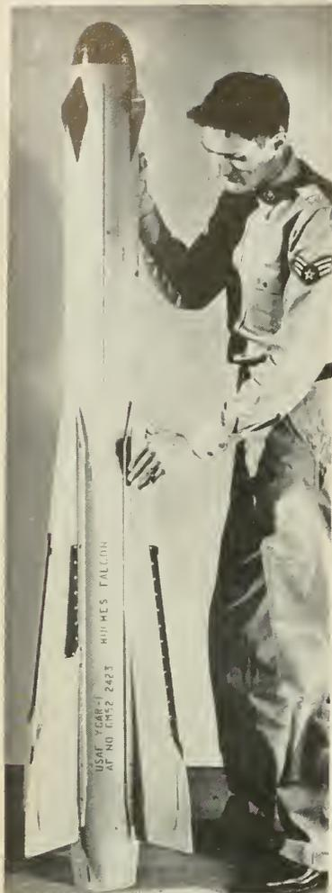
FALCON aerodynamic configuration is termed pseudo-canard. The forward wings are fixed with steering accomplished by control surfaces placed at trailing edge of stabilizers.
