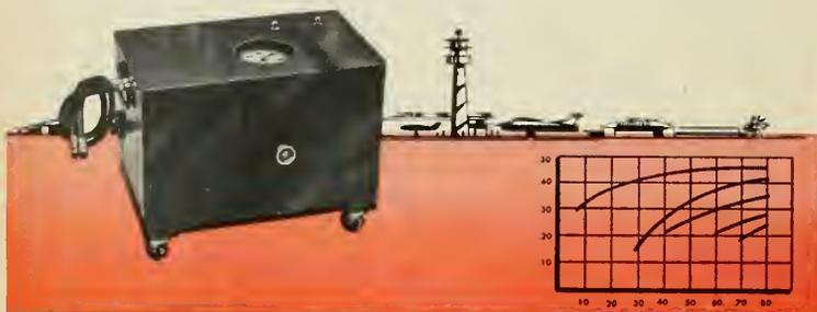
This unit is explosion proof and features a demand system with constant pressure to 3000 psi. Pressure is accurately adjustable to 25 psi, the system is filtered and is powered by a piston-type, air-hydraulic booster pump incorporating an automatically operated air selector valve. All parts are commercially available.
