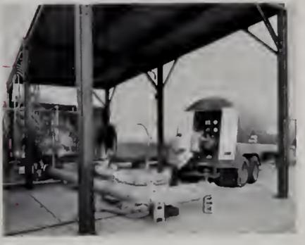
Pressure transfer evaluation using 300 PSI Liquid Oxygen Converter flowing into tower tank
