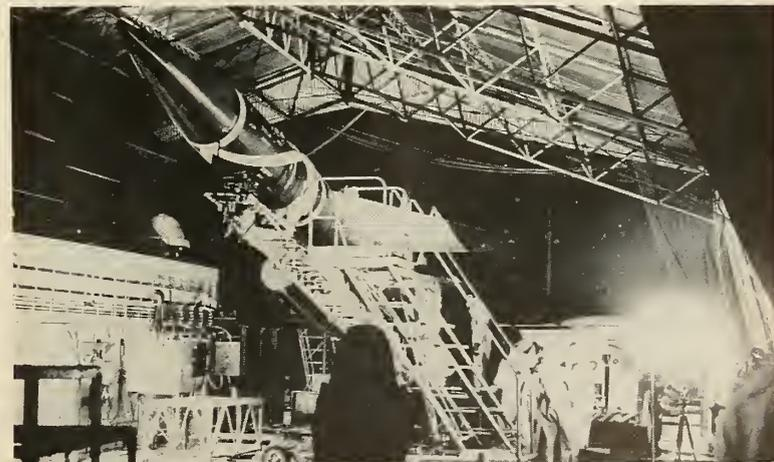
XIM-99 interceptor missile, secured to its erector-launcher, is serviced in rail-mounted field shed in preparation for launching. XIM-99 flights have been made since autumn 1952.
