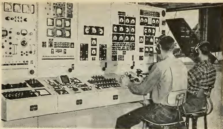
Check out of controls for *Regulus II* is conducted from this Tunny Panel, which is identical to the control system used for *Regulus* missile in submarine.
