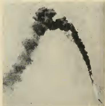
The Patrick AFB range safety officer exploded the missile because one engine failed.
