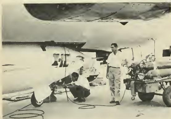
X-1E is prepared for hook-up to its B-29 mother plane. Pilot's breathing oxygen system is checked at Edwards AFB. X-1E uses advanced pilot ejection seat equipment and modified fuel feed system.
