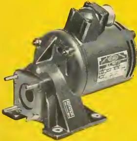
**Type:** D-899 400 cycle 3 phase AC Motor. **Weight:** 11.25 lbs. **Volts:** 200 volts. **Load:** 2.75 hp continuous output. **RPM:** 3140 rpm output at gear box. **Power factor:** 83%. **Overall efficiency:** 76% for entire unit. **Meets Military Specification MIL-M-7969A (ASG).**
