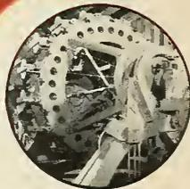
THE PLANETARY CABLE and other Roesch-developed, exclusive equipment allow O-R to fabricate cable to your individual needs.
