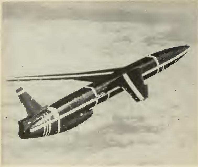
Below, Northrop's SNARK takes off from Patrick AFB at night. Two solid propellant boosters accelerate the missile from its zero-length launching rail. Missile cruises (above) at Mach 0.94. Range is 5000 miles. Warhead is delivered at supersonic speed.
