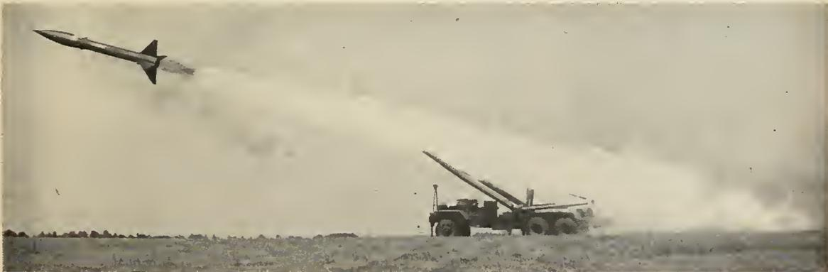
Powered by a solid propellant rocket HONEST JOHN leaves rails of launcher. A slow spin is imparted to the missile by small spin rockets.
