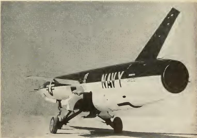
*Regulus II* test vehicle is powered by a J65 turbo jet engine. Later versions will employ the more powerful J79 power plant. This vehicle also employs boundary layer control.
