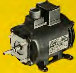
**Type:** D-800 400 cycle 3 phase AC Motor. **Weight:** 8.75 lbs. **Voltage:** 208 volts. **Horsepower:** 2.5 hp. **Continuous Duty:** 11,300 rpm; Equipped with thermal protector. **Meets Military Specification MIL-M-7969A (ASG).**
