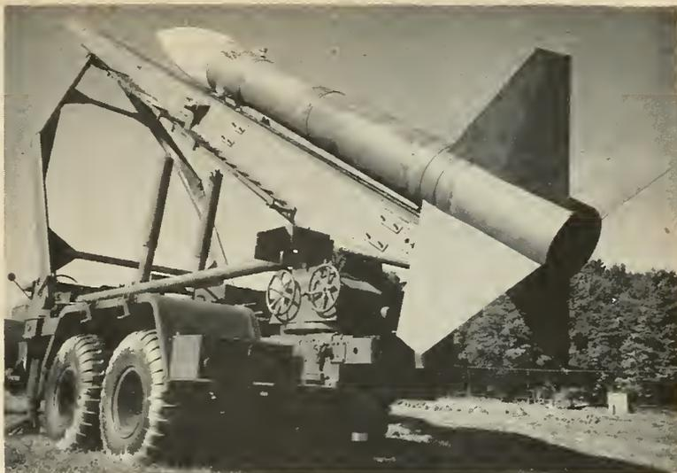
HONEST JOHN positioned on rails of its self-propelled launcher in preparation for firing.
