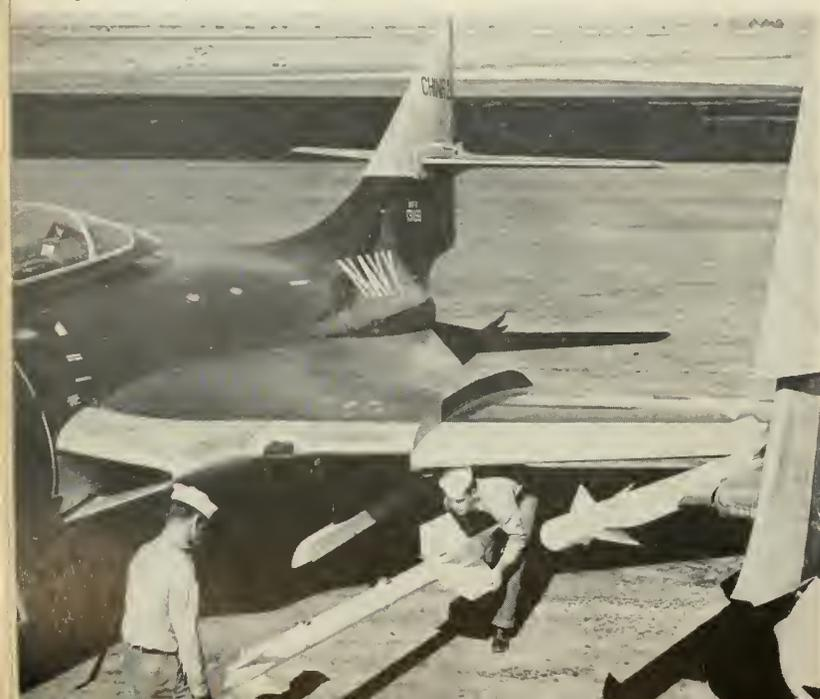
inches long, has a nozzle 7 inches long with 3-inch inside diameter. Burning time is 2 seconds.
