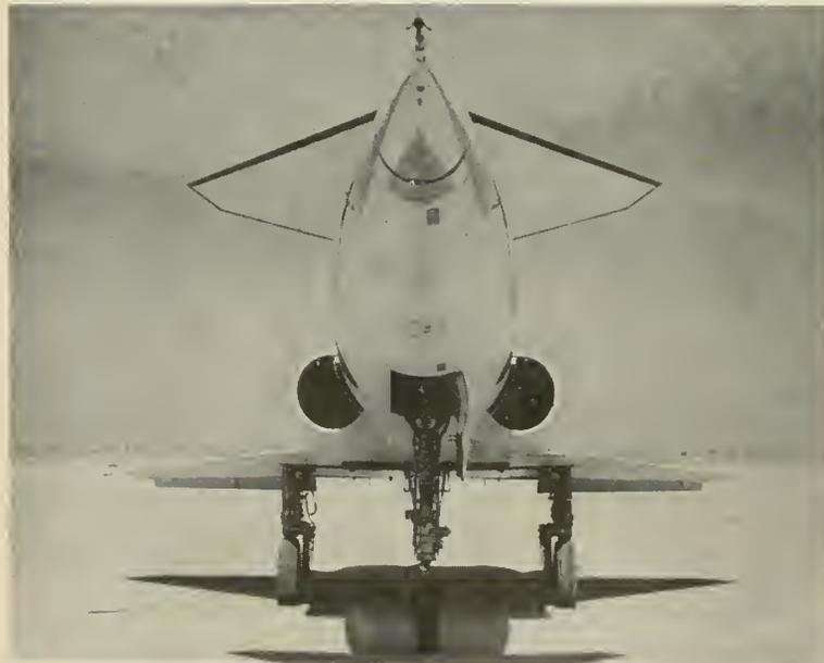
X-10, North American Aviation's unmanned test vehicle for AF's SM-64 NAVAHO intercontinental strategic aerodynamic cruise missile has concluded its flight test program. Launched by rockets and powered by turbojets, X-10 has provided much valuable research and development data for other missile programs. NAVAHO will use modern ramjet sustainers,
