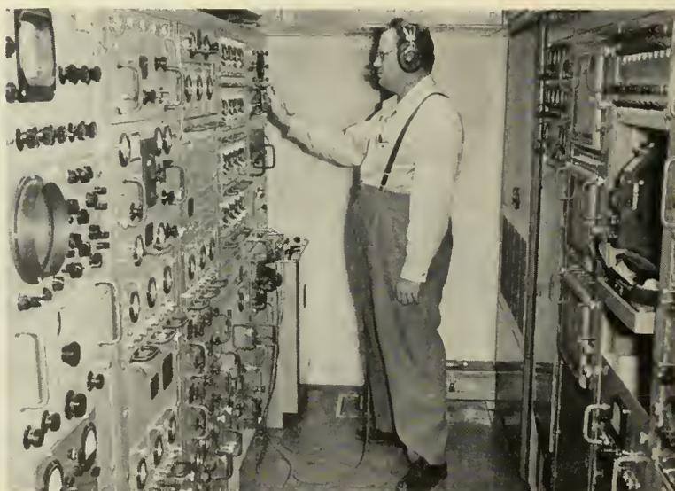
Telemeter van used for checking telemeter gear in Regulus II during flights. Regulus II has flown at more than 1½ times the speed of sound and above 50,000 ft.
