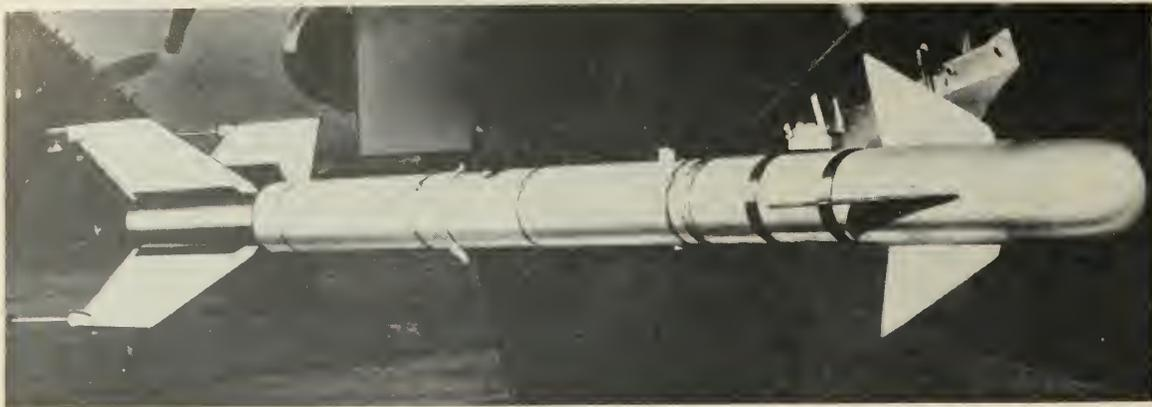
The ultimate in simplicity, Navy's **SIDEWINDER** air-to-air infrared missile, has less than two dozen moving parts and no more electronic components than an ordinary radio.
