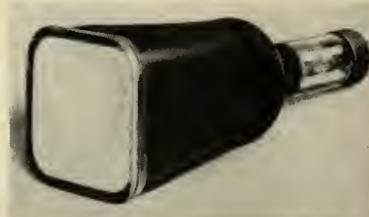
single-gun electrostatic focus and deflection cathode ray tube. Overall length is  $11\frac{1}{2}$ ". Traces are held within 1 degree of each other and deflection factor is held to within 10%. A low current gun is used.
