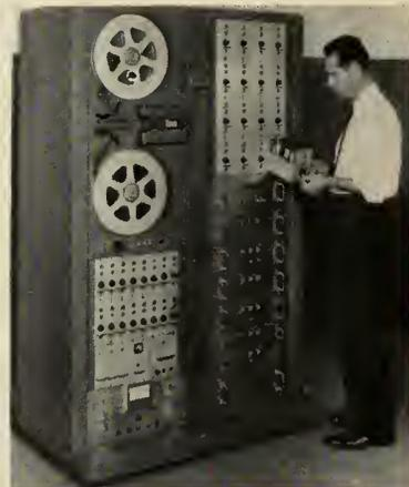
recording system. Made by the Recordata Division of American Electronics, the system accommodates reel sizes to 14" and a single switch selects one of six standard speeds up to 60"/sec.
