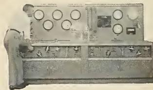
TEST STAND FOR PNEUMATIC FUNCTIONAL TESTING OF MISSILE COMPONENTS. REGULATES HELIUM FROM AN EXTERNAL PRESSURE SOURCE TO VARIOUS PRESSURE OUTLETS FROM 100 TO 3000 PSI.
