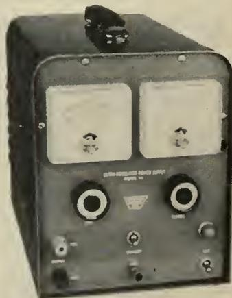
tem to achieve optimum performance consistent with light weight, compactness, and efficiency. This supply, which can produce 0 to 7 v at up to 1.5 amperes, is said to be superior to batteries in almost all applications.
