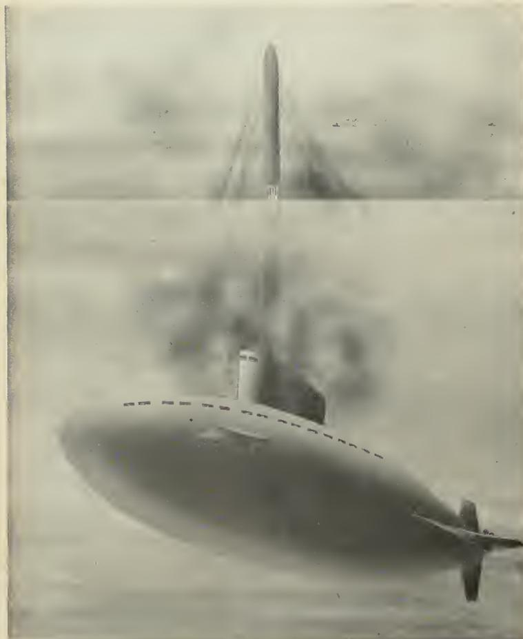
The POLARIS is described as a stubby missile with a range of 1500 miles. Special submarines using ALBACORE-type hull are understood to be planned for the Navy's fleet ballistic missile. The *Polaris* can also be launched from surface ships. Lockheed is prime contractor.
