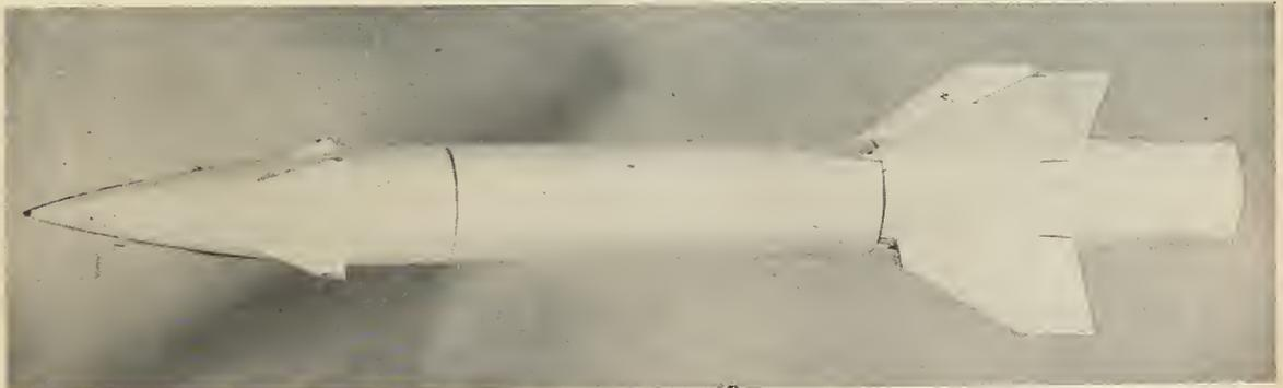
Manufacturer: Martin Co.; Range: PUP-15,000 ft., DOG-25-30,000 ft.; Speed: PUP-Mach 1.8, DOG-Mach 2; Diameter: 12 in.; Span: 12 in.; Guidance: self-contained navigation system; Powerplant: (1) Aerojet-General; Status: advanced development.
