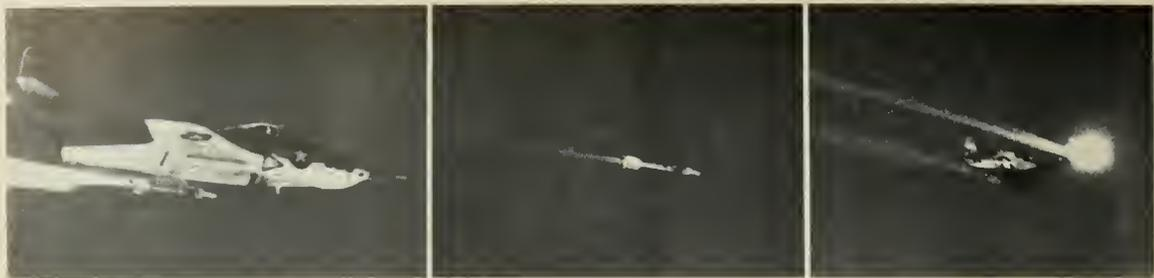
High over the Mojave desert, a Sidewinder missile is fired from a Navy jet fighter and streaks through the air for a kill against a target drone. Sidewinder is one of the most potent weapons in current use. Future versions will employ infra-red self-homing guidance.
