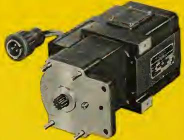
**Type:** D-927 DC Motor. **Weight:** 7.25 lbs. with 2-circuit noise filter for ungrounded systems. **Weight of filter:** 1 lb. **Terminal voltage:** 27 volts, 18 amps. **Load:** 0.5 hp. **Speed:** Continuous at 9900 rpm. **Meets Military Specification MIL-8609.**
