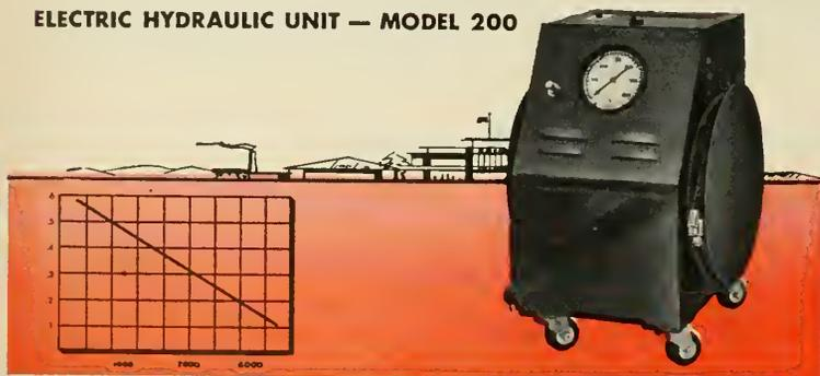
This 110V ac or dc unit features a demand system with constant pressure to 3000 psi. Pressure is accurately adjustable to 25 psi, the system is filtered and is powered by a high-speed, high efficiency gear pump. All parts are commercially available.
