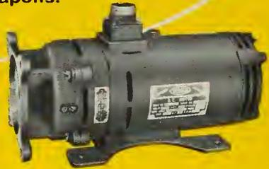
**Type:** D-638 400 cycle AC Motor. **Weight:** 17.5 lbs. **Voltage:** 200 AC, 20 amps at 6.5 hp. **Duty cycle:** 3.0 seconds at 6.5 hp, 15.0 seconds at 1.5 hp. **Maximum capacity:** 6.5 hp. **Continuous rating:** 5 hp at 2300 rpm, 15.8 amps, 200 volts. **Meets Military Spec. MIL-M-7969A (ASG).**
