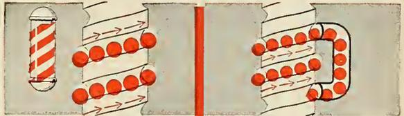
Nut glides on steel balls. Like stripes on a barber pole, the balls travel toward end of nut through spiral "funnel" formed by concave threads in both screw and mating nut.
