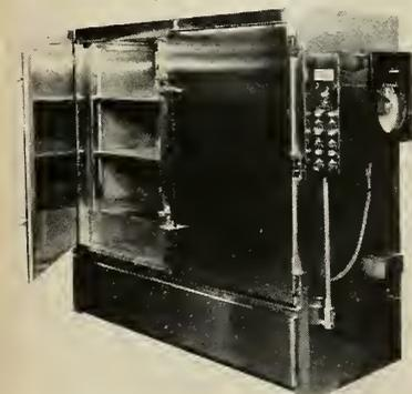
less steel, insulated with Fiberglas, perforated diffuser walls for uniform air flow, dual blowers, dual hydraulic thermostats for temperature control, silicone door gaskets, adjustable shelves.
