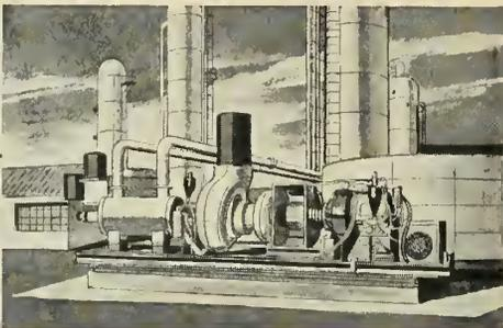
Turbine drives for gas compressors.
