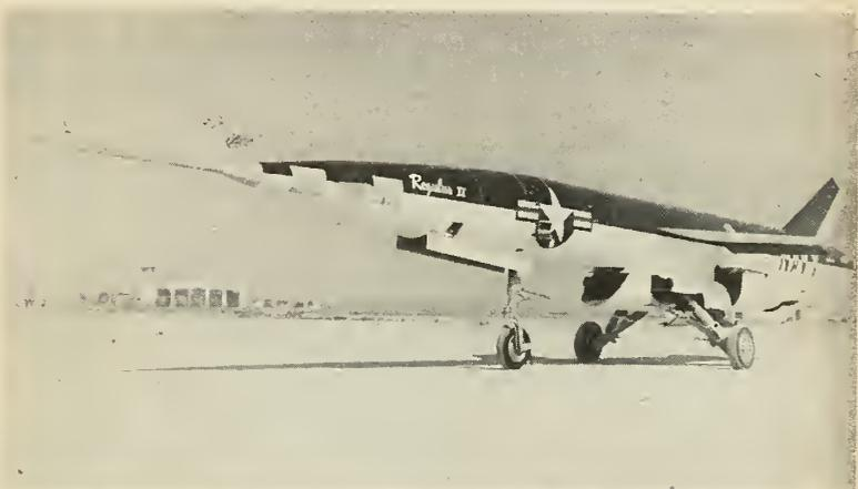
Ground view of the supersonic *Regulus II* at Edwards Air Force Base, California. Missile can carry nuclear warhead and is designed to be launched from subs as well as surface vessels.
