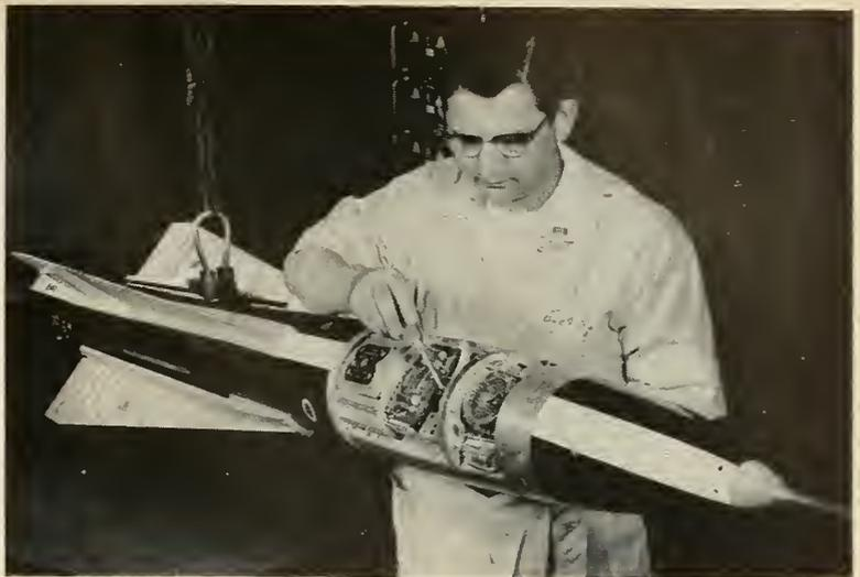
Panel removed shows BMD test bomber defense missile's circuitry for control and guidance.
