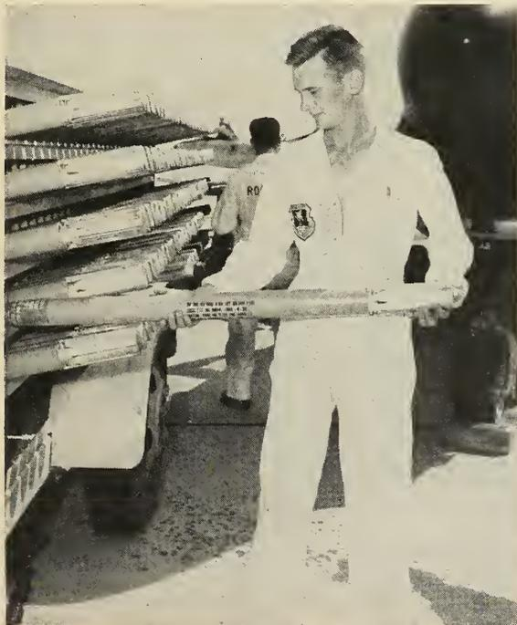
Simple missile used by the Air Force is the 2.75" MIGHTY MOUSE, standard weapon for our jet fighters. Missile is easy to handle.
