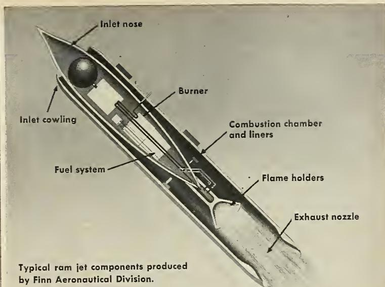
Typical ram jet components produced by Finn Aeronautical Division.
