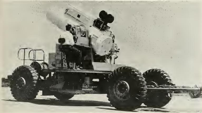
First completely mobile optical tracking system, capable of photographing an object 2" x 7" at an altitude of 4 miles, has been delivered to the Air Research & Development Command. System will soon undergo range evaluation tests at ARDC's Armament Center, Eglin AFB, Fla.
