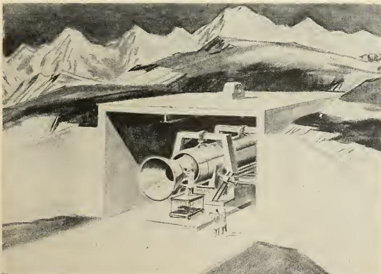
ABOVE—Artist's sketch of Thiokol's static test facilities in Utah where SERGEANT may be tested. RIGHT—The possible SERGEANT configuration superimposed on X-17 test vehicle.
