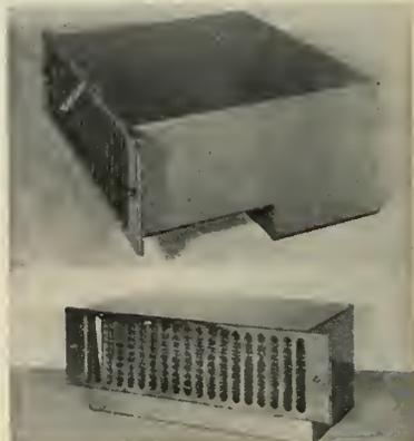
in the normally unused base section of the rack since blower is normally the bottom component of a relay rack. Models 2P408 and 2Q408 require 5 1/2 on panel height but have performance of models requiring more height. Unit will dissipate a 1.5 kw heat load with an air temperature rise of 10°C.
