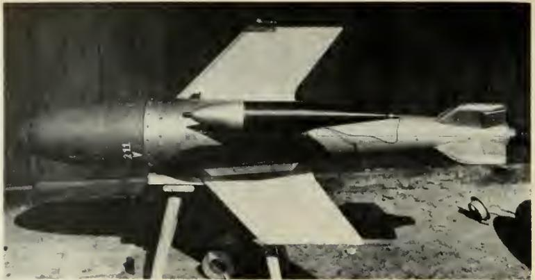
German X-4 was developed as a wire controlled, rocket propelled, gyro stabilized missile. It employed a proximity fuse. By the time World War II ended it was almost ready to use.
