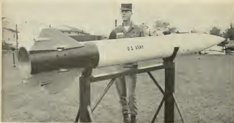
LITTLE JOHN is 12 feet long and 12½ inches in diameter. Fins are moveable and equipped for flares.
