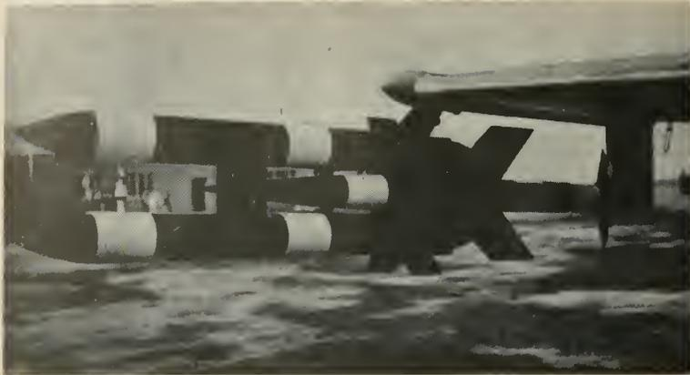
The Fairey Fireflash, first British air-to-air guided weapon to destroy radio drone. Two external boost sockets accelerate missile to supersonic speeds. It is a beam rider.
