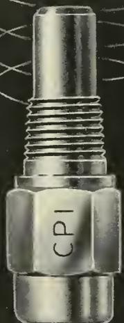
CPI PLUGSTATS provide precise thermal warning without colibration drift. Small physical size has been combined with rugged construction. Special alloy contacts assure clean make-and-break. Capable of 200°F overshoot from high or low normal setting. Available also with AN connector. Rated at ¼ ampere, 28 volts, AC or DC resistive loads. Contacts NO or NC. Weight approx. 1.5 oz.
