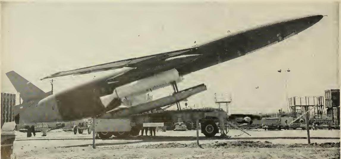
The Aerojet solid propellant boosters for the SNARK each yields 33,000 pounds of thrust. Zero-length launcher rail measures 29 feet.
