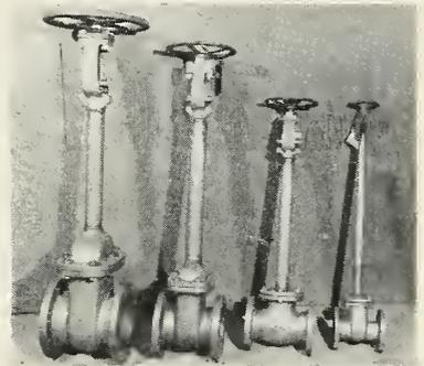
600 psi are designed with extended bonnets to permit the use of heavy insulation between the operating mechanism and the pipe line. This serves to prevent heat pick-up into the valve and its contents and to allow free movement of the operating mechanism.
