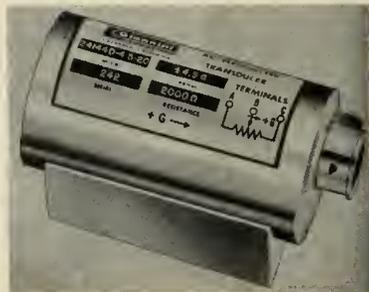
0.01g/g max. and low threshold has been developed by G. M. Giannini & Co., Inc. The units sense linear acceleration by a spring supported linear ballbushing mounted mass that moves along a shaft.
