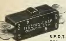
S.P.D.T., 2 circuit; 10 amps, 125/250 v. AC/ 30 v. DC. Ind. Screw or solder terminals at ends or one side of switch. Also available with reset button at bottom of switch or in Type S-100 Make-Before-Break Series where switch completes a new circuit before interrupting old one.
