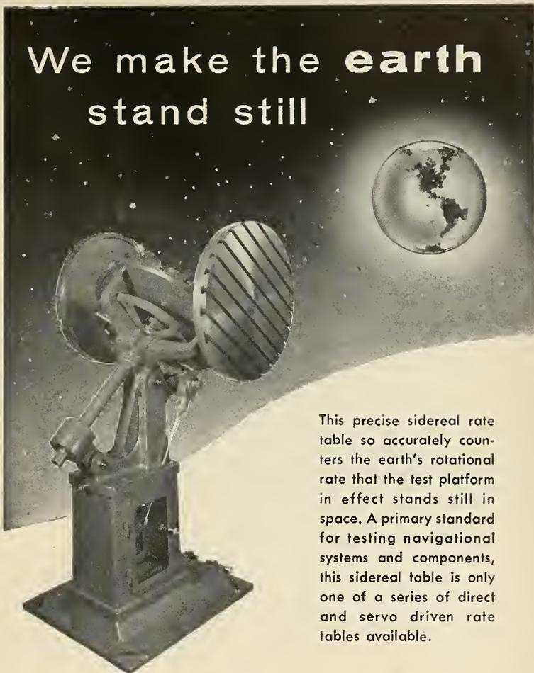
This precise sidereal rate table so accurately counters the earth's rotational rate that the test platform in effect stands still in space. A primary standard for testing navigational systems and components, this sidereal table is only one of a series of direct and servo driven rate tables available.
