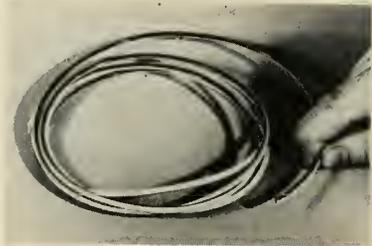
identify process lines, electrical and electronic leads. Available in any size, the tubing has good dielectric strength (500 to 1,000 v/mil); lowest dielectric constant (2.0) and dissipation factor (0.0002) of any solid dielectric; no change of electrical properties with temperature or frequency.
