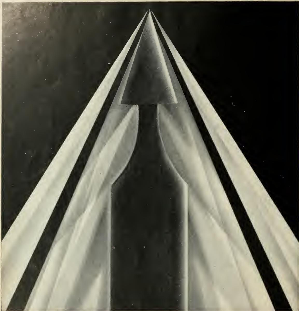
*Shock wave around a simulated missile*
