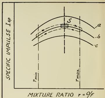
Automatic control of  $P_c =$  constant and mixture ratio = constant. a to c are curves of three different  $P_c$  values as parameters. S = area covers the tolerance for an acceptance test.
