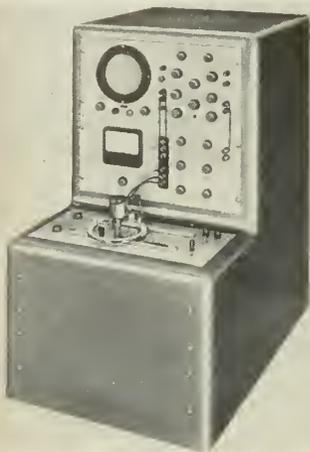
Use of a long persistent oscilloscope provides display of error signal, and noise due to contact resistance over frequency range of 0 to 100,000 cycles. Individual wire commutation may be shown. Magnetic clamping allows rapid set-up and alignment of test potentiometers.
