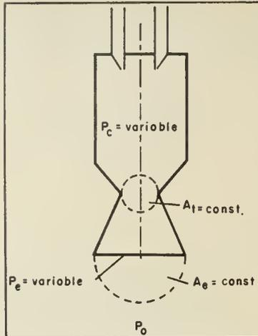
Parameters of a fixed expansion nozzle.
