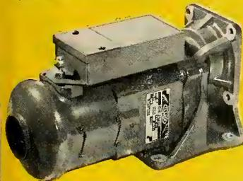
Type: D-751 DC Motor. Weight: 20 lbs. Duty Cycle: 5.2 hp at 2100 rpm (intermittent) on 26 volts DC; 3.5 hp at 2200 rpm (continuous) on 26 volts DC. Meets Military Specification MIL-M-8609.
