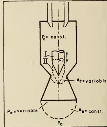
Parameters of a variable expansion nozzle.
