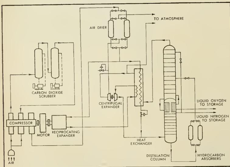
Flow diagram of 75 T/D LOX Generator. It's said to cut big quantity production rates to about .7¢ per pound of LOX and liquid nitrogen. Designed to run by electric power.
