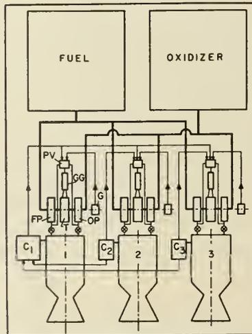
High thrust powerplant applying three combined rocket units. The master controller  $C_1$  of unit 1 mixes the signals received from the other controllers  $C_2$  and  $C_3$  and compensates for the deviation according to the thrust set valve. Separate governor control loops are required to maintain stable conditions during starting transient. (PV = prop. valve; GG = gas generator; T = turbine; FP = fuel pump; OP = oxidizer pump; G = governor.)
