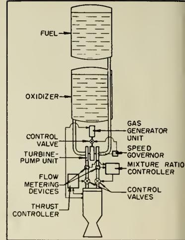
Rocket powerplant with turbine/pump-unit including automatic thrust and mixture ratio control.
