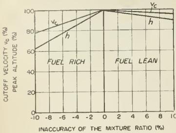
Loss of cut-off velocity and peak altitude, respectively, due to the inaccuracy of the mixture ratio using the propellant combination C(NO<sub>2</sub>)/JP-4.
