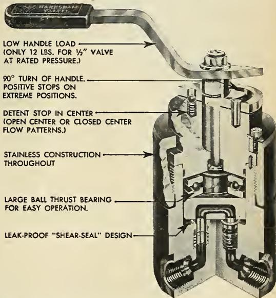
This new four-way valve series comes in pipe sizes from 1/4 to 1 inch, but may be obtained with tube, AND 10050, or any preferred special high pressure connection. It will withstand surges of up to 15,000 P.S.I. without damage to the valve's sealing qualities. It is designed for a burst pressure of 30,000 P.S.I.
