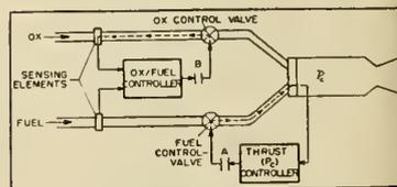
Test arrangement for the stability investigation of a bi-propellant rocket powerplant with a thrust and mixture ratio control loop. At A and B the loops can be cut for investigation purposes.
