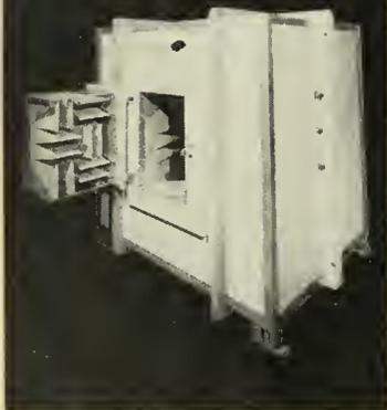
Portable test chamber as shown (Size 65" x 54½" x 65") and designed for a low-frequency cut-off at 250 cps. Chamber is mounted on Korund spring vibro-isolators.
