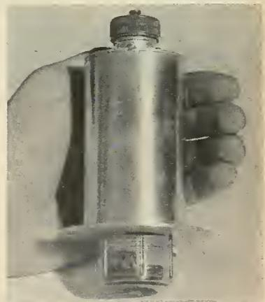
programming devices and explosive element initiation. The unit provides for a settable time delay between 0.3 and 10 seconds, with an accuracy of  $\pm 5\%$ , and output energy in excess of 35,000 ergs. Temperature ambients from  $-70^{\circ}\text{F}$  to  $165^{\circ}\text{F}$  and accelerations up to  $100\text{ g's}$  have no effect on the device, which is termed the PM-47.
