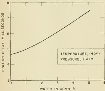
Table showing overall effect of water in UDMH on ignition delay with IRFNA.
