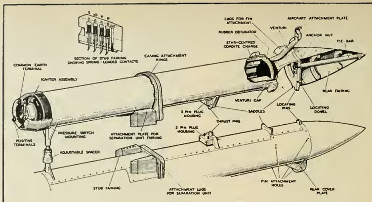
Cut-away view of FIREFLASH booster rocket and attachment fittings.
