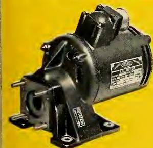
Type: D-899 400 cycle 3 phase AC Motor. Weight: 11.25 lbs. Volts: 200 volts. Load: 2.75 hp continuous output. RPM: 3140 rpm output at gear box. Power factor: 83%. Overall efficiency: 76% for entire unit. Meets Military Specification MIL-M-7969A (ASG).
