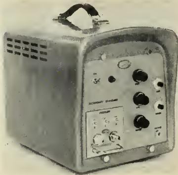
direct pressure measurements is being introduced by Wianco Engineering Co. The portable, compact unit has an overall accuracy of  $\pm 0.05\%$  of full-scale ranges of 5 psi to 2500 psi, and  $\pm 0.1\%$  for ranges of 3000 psi to 10,000 psi.
