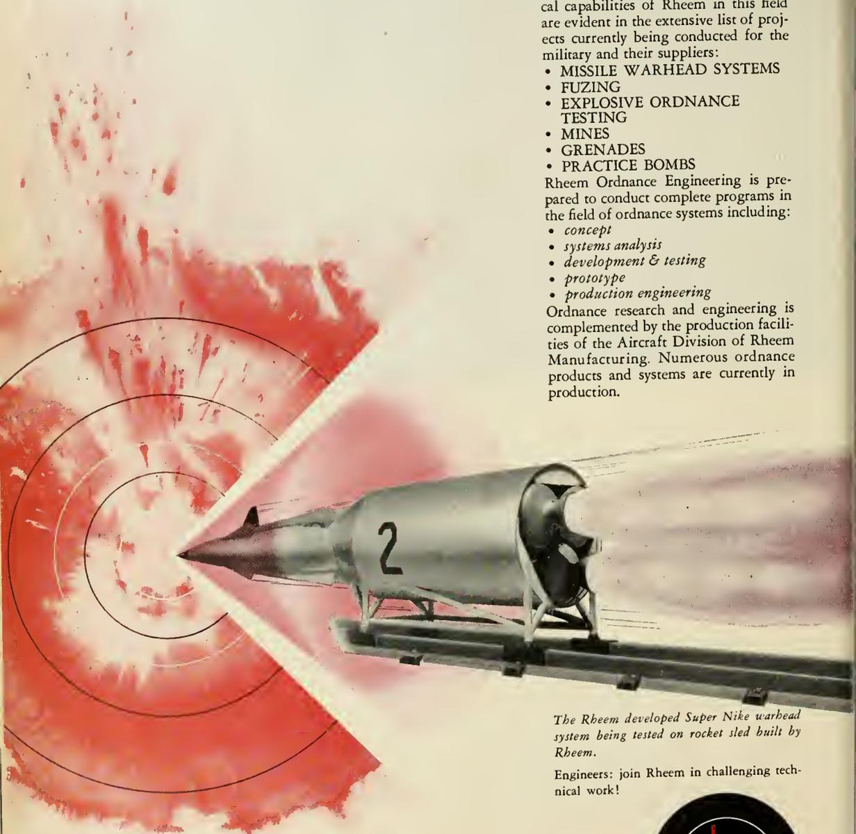
*The Rheem developed Super Nike warhead system being tested on rocket sled built by Rheem.*
