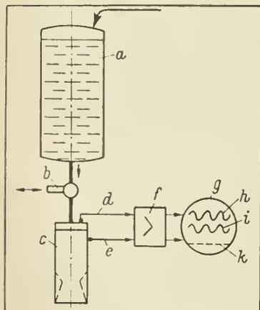
Test arrangement for the stability investigation of a mono-propellant pressurized system. (a) propellant tank (b) piston pulser to generate a harmonic disturbance (c) combustion chamber (d) injection pressure  $P_i$  (e) chamber pressure  $P_c$  (f) amplifier (g) oscillograph (h)  $P_c$  as the input variable (j)  $P_c$  as the output variable (k) time mark.
