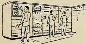
This ASCOP PW Ground Station is a complete "packaged" system for data processing. Eighty-six Channels may be reduced in real time from tape records. Utilization of zero and full scale sensitivity reference channels affords continuous automatic system calibration, avoiding frequent manual adjustment and the need for critical components. All channels may be visually monitored simultaneously. Easy access to slide mounted chassis is featured even during operation.
