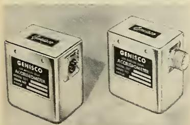
in the Genisco model DDL accelerometer now in production. The new configuration is designated the model DDT and embodies a pair of miniaturized solenoids which permit either pre- or in-flight simulation of full-scale operational accelerations by displacement of the sensory mechanisms.
