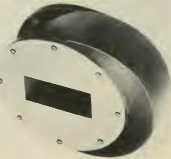
The resonant absorption isolators furnish constant uni-directional magnetron to load isolation and feature a waveguide size of 2.00 x 1.00 O.D. with a weight of less than 3.5 lbs. Electrical characteristics guarantee an isolation of 10 db minimum, insertion loss of 0.5 db maximum, input VSWR 1.10 maximum with matched load and power handling capabilities of 150 kw peak power with 100 watts average into a 2 to 1 mismatch.
