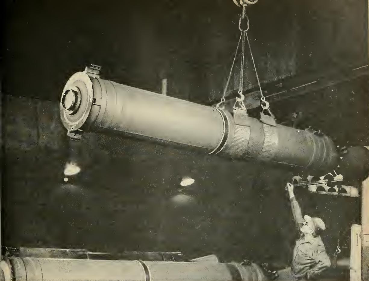
HONEST JOHN, complete except for propellant, warhead and fins, is built of steel by ALCO under prime contract.
