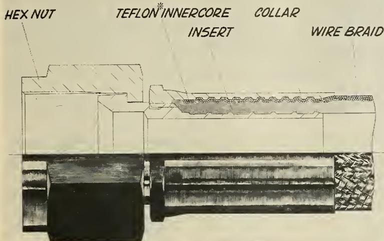
As shown in the figure, the hose is retained between an insert and a collar. Originally a loose fit over the wire braid, the collar diameter is reduced a predetermined amount by radial pressure applied progressively along its length in a rotary hydroforming machine. The plastic innercore and the braid are worked forward toward the hex nut, resulting in a
