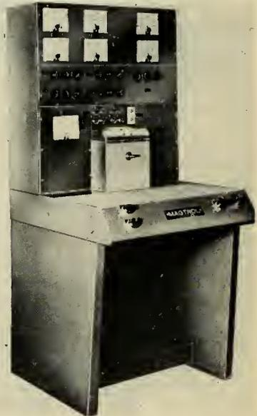
tested in a new test stand developed by Magtrol, Inc. The test stands are designed to completely test a motor in three or more dynamic phases of torque, speed and current characteristics and feature four-digit electronic tachometers to indicate motor speed.
