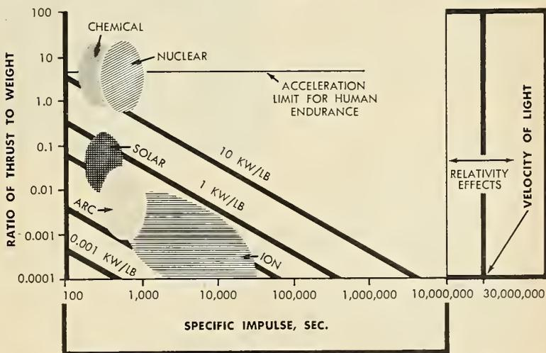
Ratio of thrust to weight versus specific impulse, sec., of different propulsion systems.
