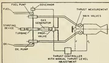
Thrust control system of a bi-propellant pumped powerplant with gas generator control for thrust level adjustment with the chamber pressure  $P_c$  as the control variable (dashed line: using thrust  $F$  as the control variable).
