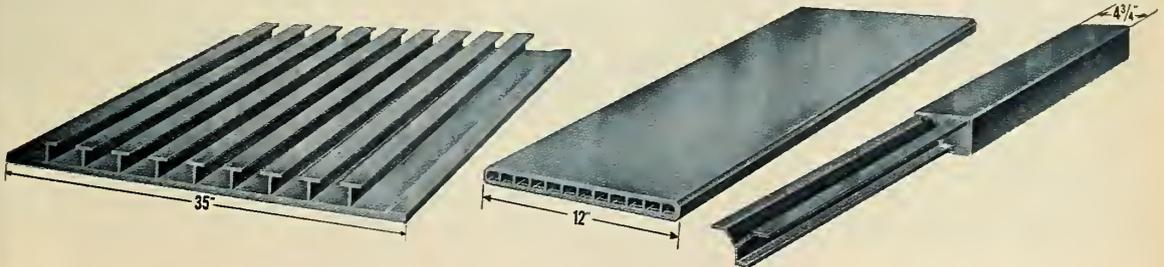
**INTEGRALLY STIFFENED SKIN PANEL** is produced in extra wide widths on heavy presses. Combination of skin and stiffeners in large panels minimizes machining, simplifies assembly, improves performance of aircraft, missiles, and military vehicles.
