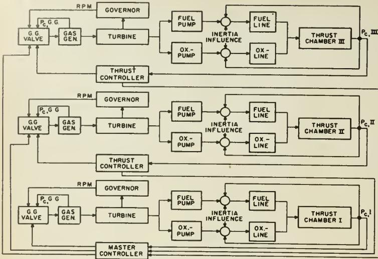
Block-diagram of the high thrust powerplant according to Fig. 8 with several "internal" loop actions and cross-connections. Probable mixture ratio control is disregarded.
