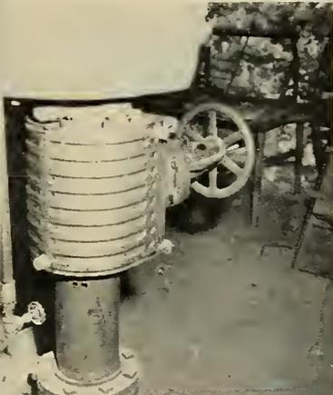
The device is made of two sheets of metal, with the outside sheet embossed to create flow channels. The inside sheet, which is flat, provides greater heat-transmitting contact. The two sheets are welded together and curved to fit the valve.
