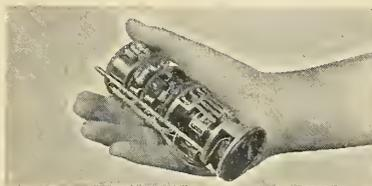
Miniaturization provides a 2" diam. x 6" long self-contained unit. (Unit is shown with case removed.)
