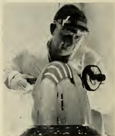
A ballistic missile test nose cone, with one of the smoothest surfaces created by man, has super buffing and polishing prior to flight into the ionosphere on the Air Force's X-17 re-entry rocket. The AF said the X-17 has brought many ballistic missile test nose cones past the extreme re-entry temperatures.
