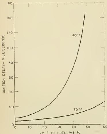
Ignition delay of JP-4/UDMH mixtures with IRFNA showing delay in milliseconds.
