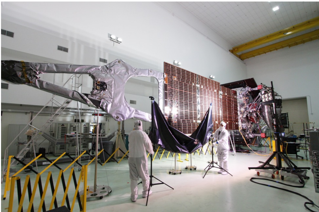
Technicians test Juno's solar arrays in preparation for launch at NASA's Kennedy Space Center. Credit: NASA
