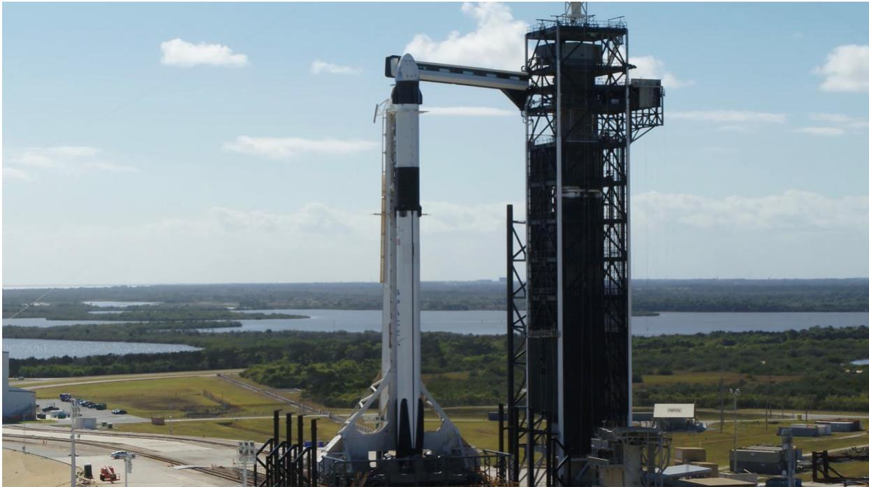
Falcon 9 is a two-stage rocket designed and manufactured by SpaceX for the reliable and safe transport of satellites and the Dragon spacecraft into orbit. Falcon 9 is the first orbital class rocket capable of reflight.
