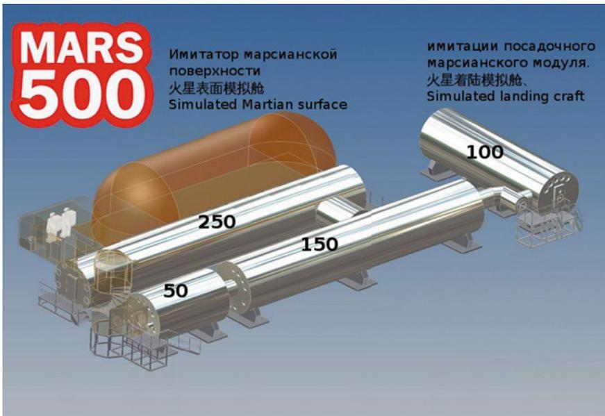
The Mars-500 module complex installed in the IBMP installation with five modules for habitat (150 and 50), medical (100), utility (250), Mars lander and Mars surface. *Credit IBMP*
