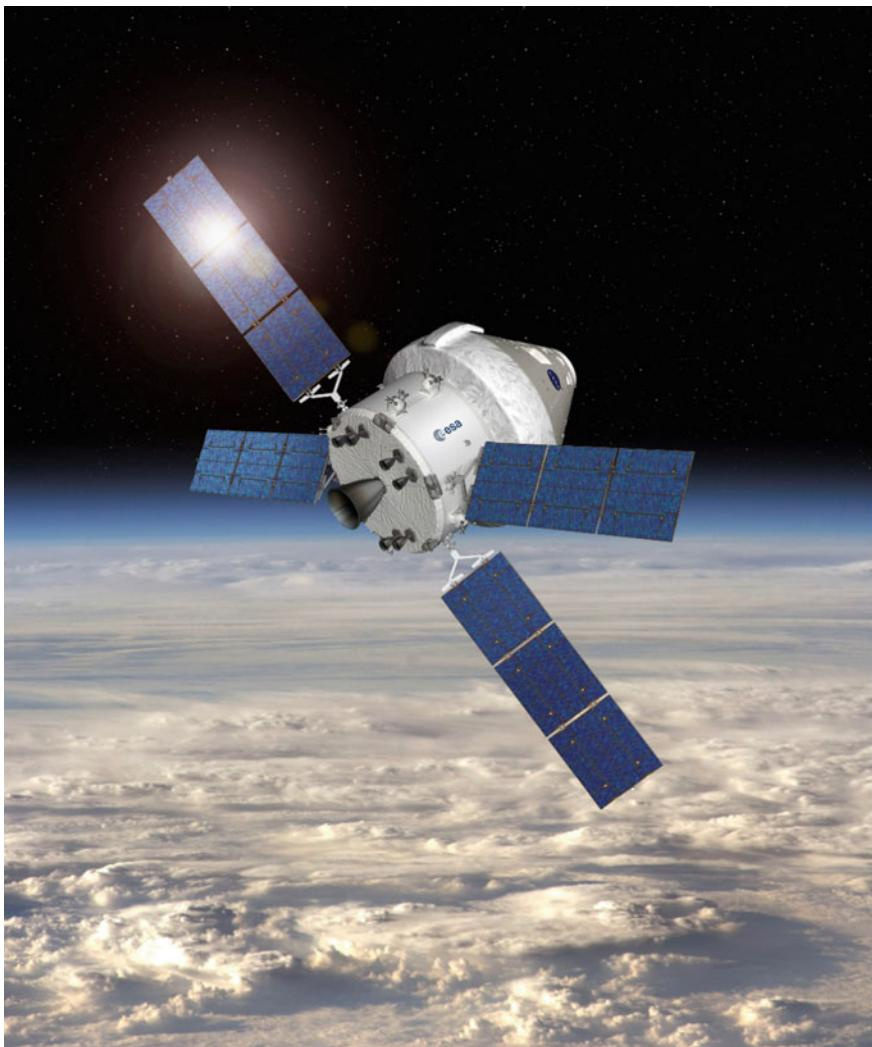
An artist's impression of the Orion spacecraft with ESA's service module. The module sits directly below Orion's crew capsule and provides propulsion, power, thermal control, and water and air for four astronauts. The solar array spans 19 m and provides enough power to power two households. A little over 5 m in diameter and 4 m high, it weighs 13.5 tonnes. The 8.6 tonnes of propellant will power one main engine and 32 smaller thrusters. *Credit ESA—D. Ducros*
