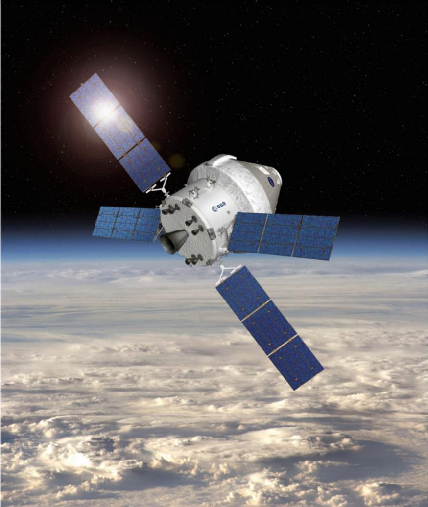
An artist's impression of the Orion spacecraft with ESA's service module. The module sits directly below Orion's crew capsule and provides propulsion, power, thermal control, and water and air for four astronauts. The solar array spans 19 m and provides enough power to power two households. A little over 5 m in diameter and 4 m high, it weighs 13.5 tonnes. The 8.6 tonnes of propellant will power one main engine and 32 smaller thrusters. *Credit* ESA—D. Ducros
