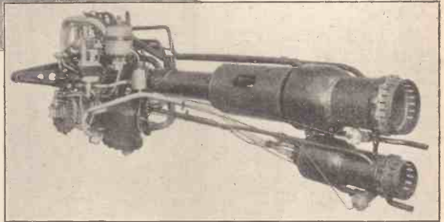
The Walter 109/509C developed for the Ju.263. Its main chamber produced a thrust ranging from 220 to 4,400lb., and an additional 880lb. constant was forthcoming from the smaller "cruising" chamber. (See PRACTICAL MECHANICS, Sept., 1946, p. 420.)
