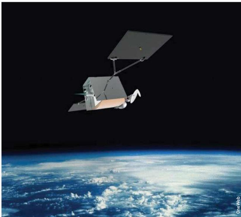
◀ OneWeb satellites will be mass produced using fewer components and lighter weight, making them easier to manufacture and cheaper to launch. They will include state-of-the-art onboard GPS sensors and on-board propulsion systems to help avoid orbital debris and for end of life disposal.
