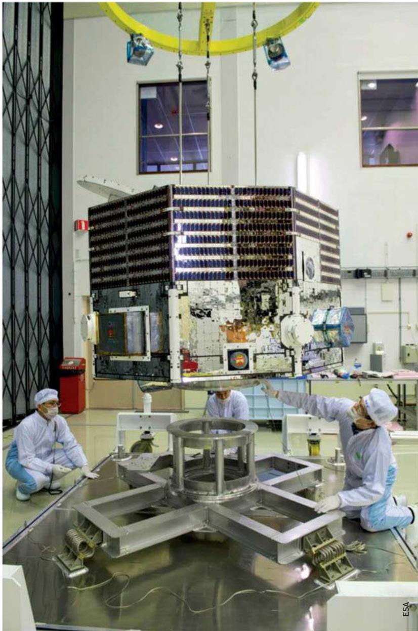
ESA is also building the Mercury Transfer Module (MTM), which will carry the two orbiters from Earth to Mercury. Upon arrival, the transfer module will be jettisoned and the two orbiters will separate.
