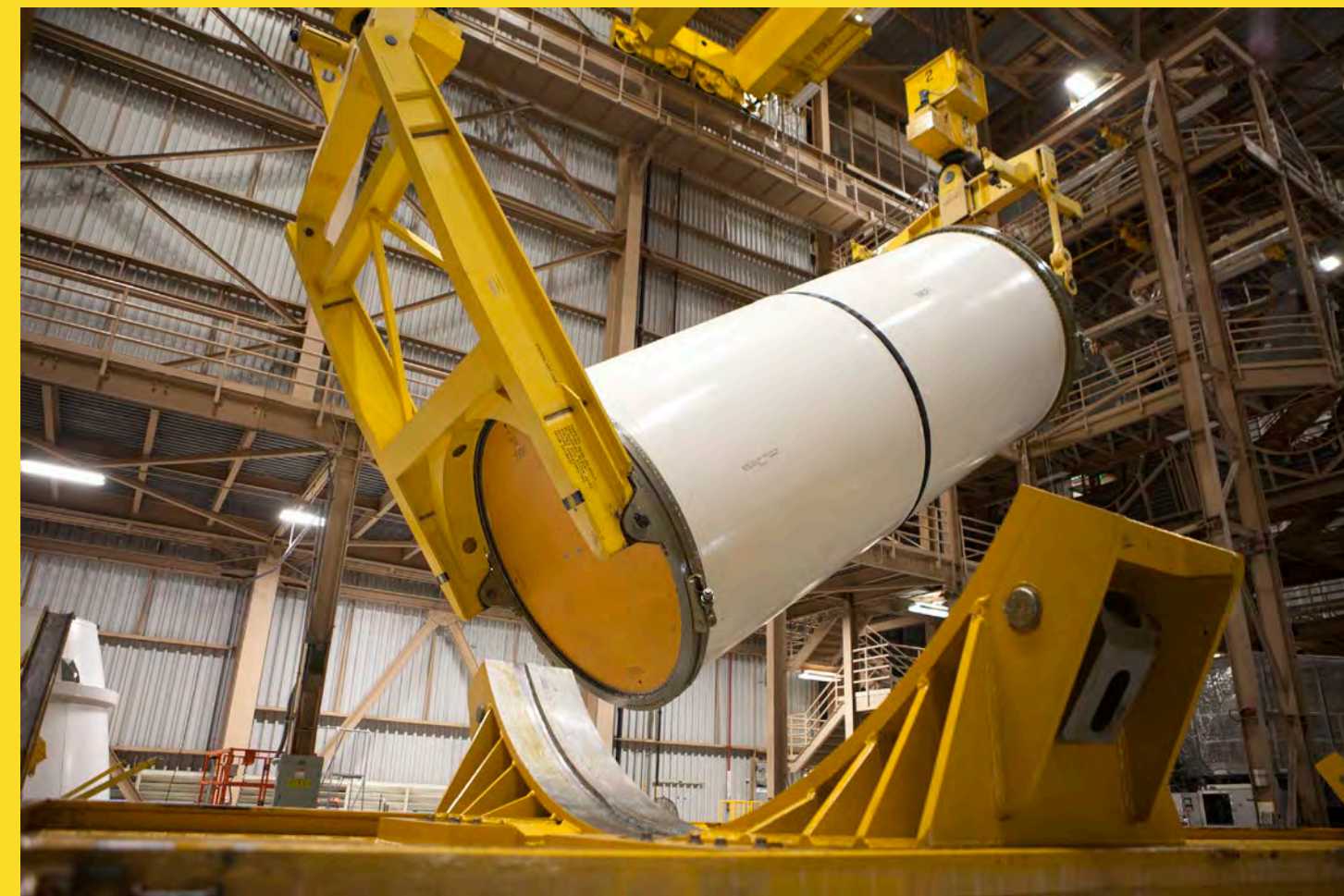
Two cranes are used in tandem to lift the first of two pathfinders, or test versions, of solid rocket booster segments for NASA's Space Launch System rocket away from a railcar inside the Rotation, Processing and Surge Facility high bay at Kennedy Space Center on Feb. 25. The booster segment will be raised into the vertical position. The Ground Systems Development and Operations Program and Jacobs Engineering, on the Test and Operations Support Contract, are conducting a series of lifts, moves and stacking operations using the booster segments, which are inert, to prepare for Exploration Mission 1, deep-space missions and the journey to Mars. The pathfinder boosters arrived at Kennedy from Orbital ATK in Utah aboard an Iowa Northern train contracted by Goodloe Transportation of Chicago. Photo credit: NASA/Ben Smegelsky
