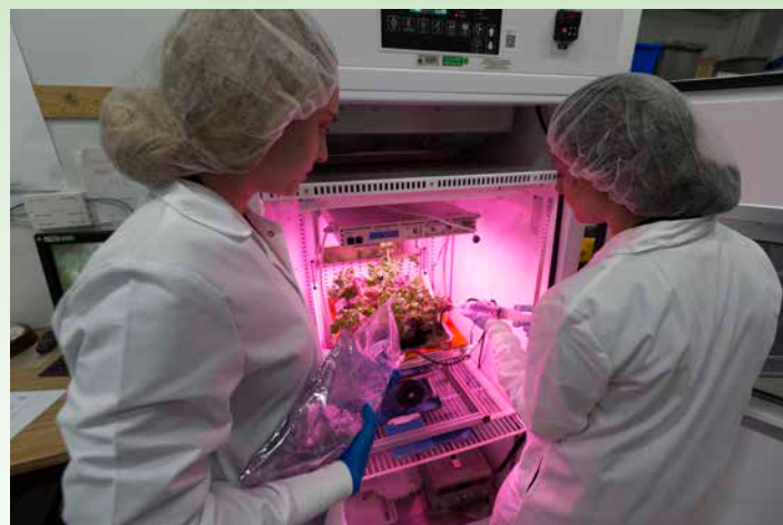
NASA interns Jessica Scotten, left, and Ayla Grandpre water plants in the Veggie hardware in Kennedy Space Center's ISS environment simulator chamber. Mizuna mustard, Outredgeous lettuce and Waldmann's green lettuce are growing in Veggie. Photo credit: NASA/Cory Huston
