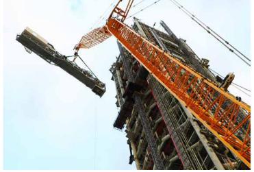
A crane lifts the Orion crew access arm so it can be attached to the mobile launcher at NASA's Kennedy Space Center. The crew access arm is designed to rotate from its retracted position and line up with Orion's crew hatch. The arm will provide entry and emergency egress for astronauts and technicians into and out of the Orion spacecraft. Photo credit: NASA/Bill White
