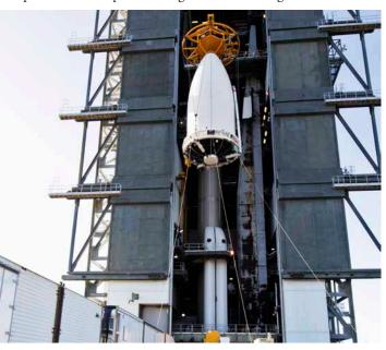
The payload fairing containing NOAA's Geostationary Operational Environmental Satellite-S (GOES-S) is lifted up by crane Feb. 16, 2018, at the United Launch Alliance Vertical Integration Facility at Space Launch Complex 41 at Cape Canaveral Air Force Station. Photo credit: NASA/Glenn Benson
