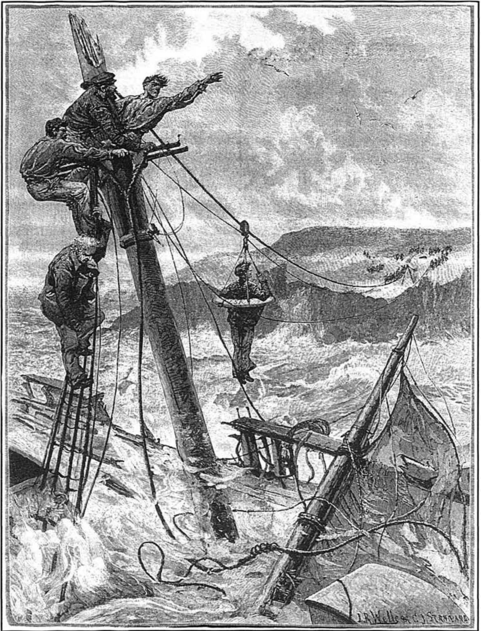
Fig. 6. Lieutenant Kisbee's Sling Life Buoy or Petticoat-breeches – Breeches Buoy in action. ( The Illustrated London News , 1886)
