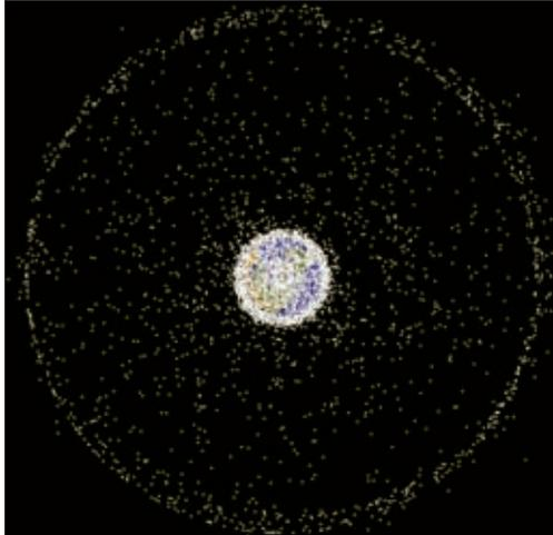
This NASA image was generated from a distant oblique vantage point to provide a good view of the object population in the geosynchronous region (around 35,785 km altitude). Note the larger population of objects over the northern hemisphere is due mostly to Russian objects in high-inclination, high-eccentricity orbits.
