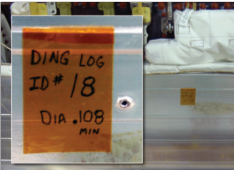
During STS-115, micrometeoroid orbital debris struck the shuttle Atlantis and left a 0.108-in. ding in its right-hand payload bay door radiator. Credit: NASA.
