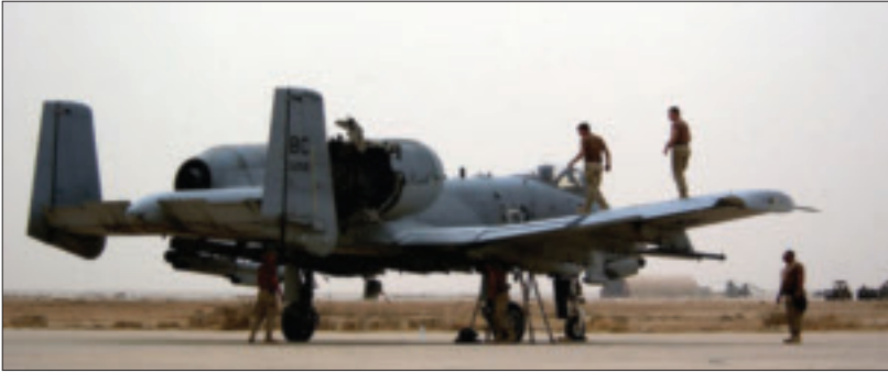
During Operation Iraqi Freedom, A-10 maintenance members from the 392 Air Expeditionary Wing inspect their aircraft for any additional damage after it was hit by an Iraqi missile in the right engine. The A-10 made it back to the base safely. USAF photo/Staff Sgt. Shane A. Cuomo.
