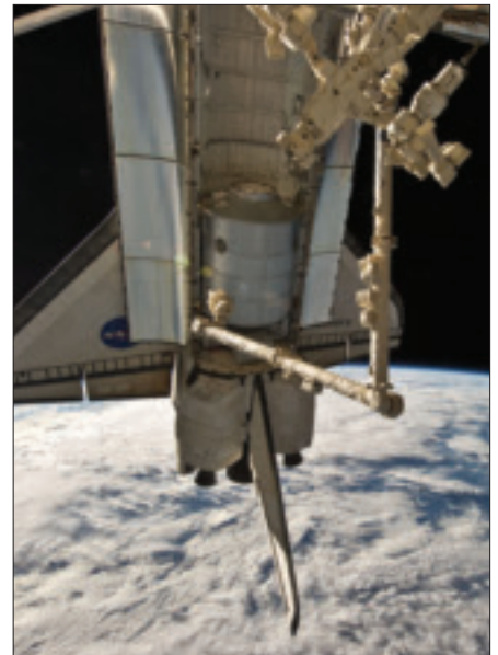
Canadarm2 grapples the Leonardo MPLM from Discovery's payload bay for relocation to a port on the Harmony node of the ISS.
