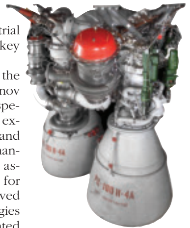
A modified RD-180 engine will serve as the first stage booster for the Rus-M family.
