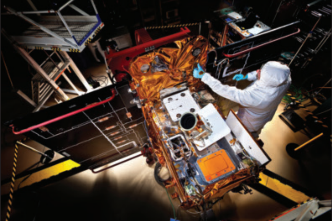
A technician checks the bottom side of a solar panel, revealing the colorful internal components of the spacecraft. The horn-shaped feature at the center is the swiveling star tracker. Credit: Lockheed Martin.
