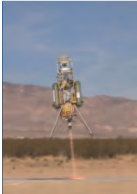
Xombie performs a vertical takeoff/vertical landing test flight. Photo courtesy Masten Space Systems.
