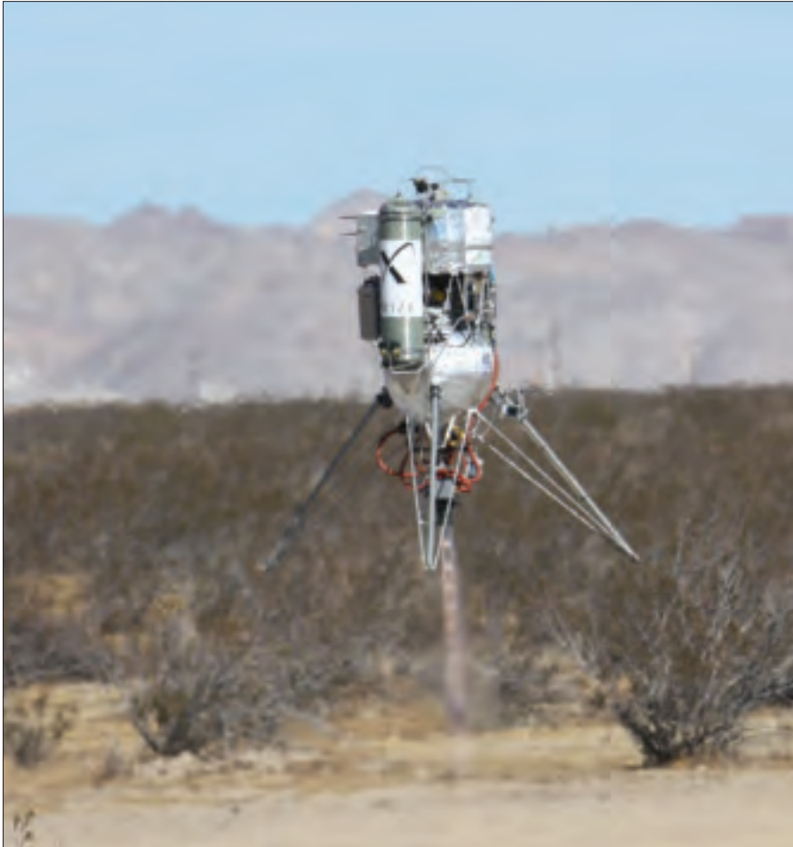
Masten Space Systems XA0.1E rocket, nicknamed "Xoie" (pronounced Zoey) hovers under rocket thrust at the Mojave Air and Space Port in California. Kluft photo.
