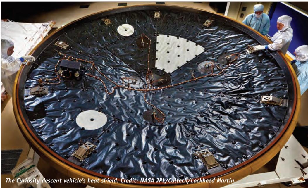
The Curiosity descent vehicle's heat shield. Credit: NASA JPL/Caltech/Lockheed Martin.
