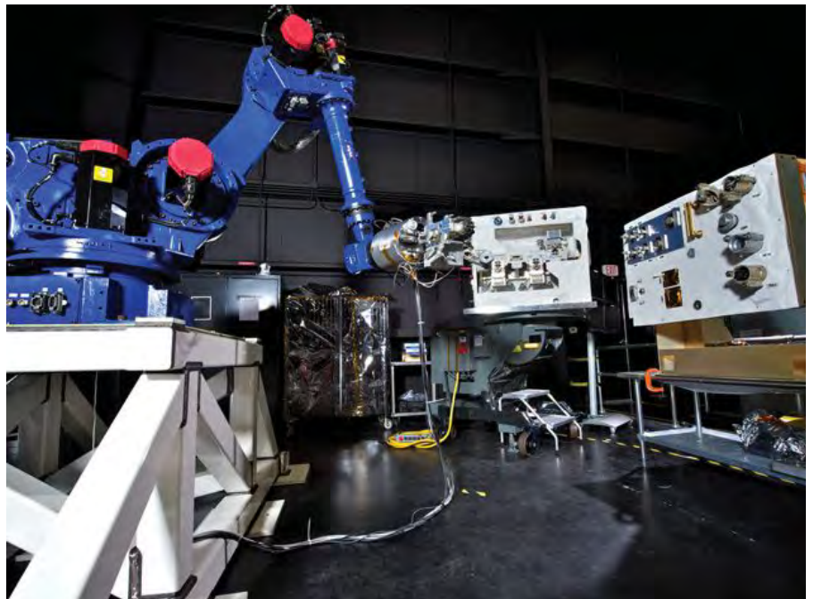
In ground tests, a robot practices robotic refueling missions on mock satellites. Credit: NASA.
