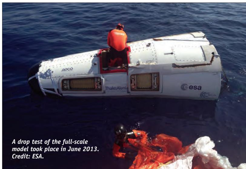
This marked the genesis of the Intermediate Experimental Vehicle, initiated as part of ESA’s Future Launcher Preparatory Program in 2004. According to Quaglino, following “a thorough industrial trade-off on shape and system concepts...the concept selected for the IXV was a lifting re-entry body,” designed for launch by ESA’s Vega rocket on an equatorial trajectory leading to re-entry and parachute-assisted splashdown in the Pacific Ocean about 100 minutes later.
