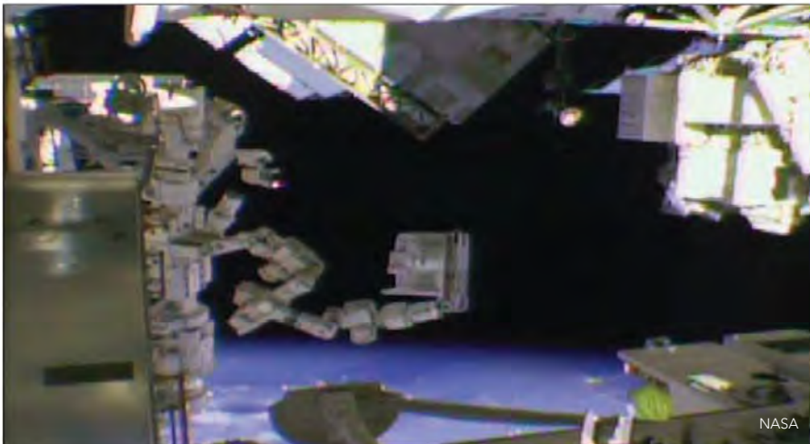
Canada's two-armed Dextre robot was photographed installing the Optical Payload for Lasercomm Science on the space station exterior.
