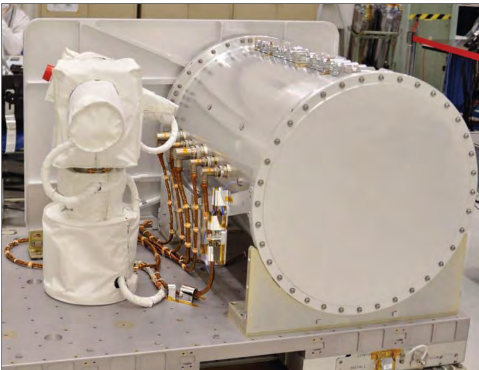
The electronics and laser for OPALS, the Optical Payload for Lasercomm Science, are protected by a cylindrical housing. The gimbal that steers OPALS is to the left.
