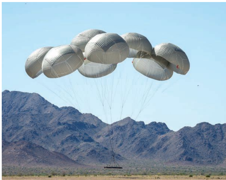
▲ A 19,000-kilogram test of a cluster of eight G-16 parachutes. U.S. Army
